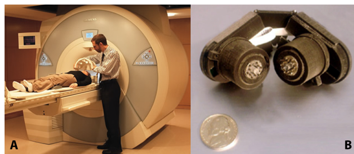
Figure 4: A: A fMRI machine B: The latest version of the OTIS system developed by Archinoetics (fNIRS) (slightly modified from [36, 93]).
