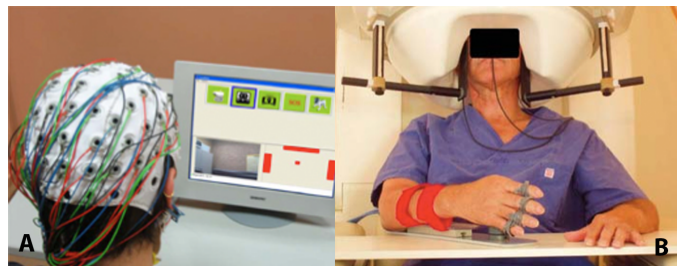
Figure 3: A: A scalp EEG based BCI system controlling different electrical devices B: A BCI system controlling a flexible hand prosthesis based on MEG (slightly modified from [11, 24]).
