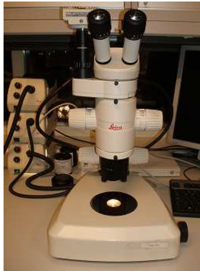
Figure 7: The Leica MZ 9.5 stereomicroscope connected to a camera, for capturing images of the sectioned otoliths.
