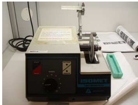
Figure 5: The Isomet 1000 low speed saw, with a block of hard epoxy resin containing otoliths to be sectioned attached. To the right is a rubber mould used for embedding.
