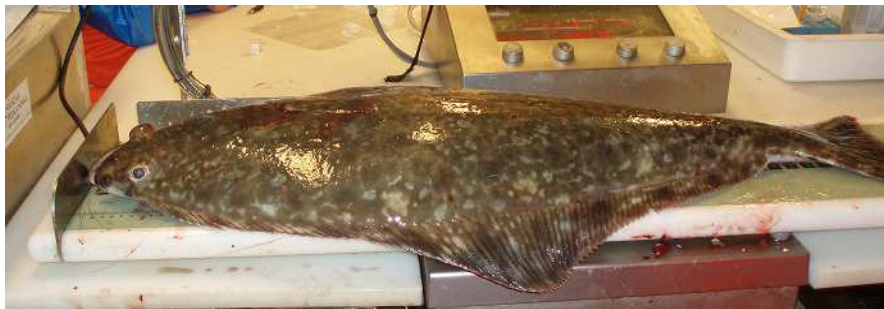
Figure 3: The total length of a halibut measured on a fish meter® (Scantrol).
