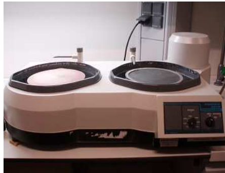
Figure 6: The Buehler Phoenix beta rotating disk used for grinding and polishing.
