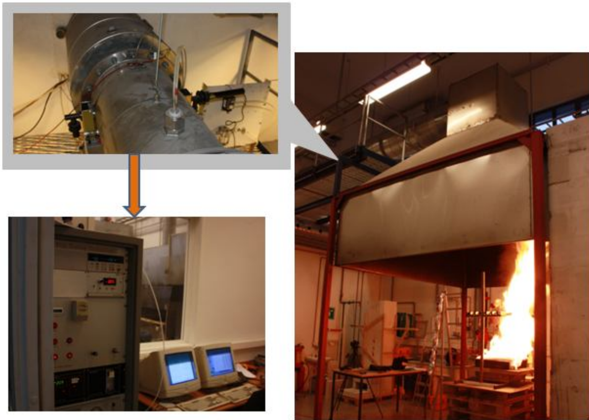
Figure A-4 Cone calorimeter with analysing equipment
