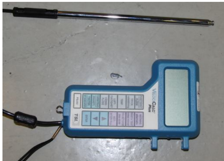
Figure A-3 VelociCalc Plus Meter (Model: 8386-M-S)
