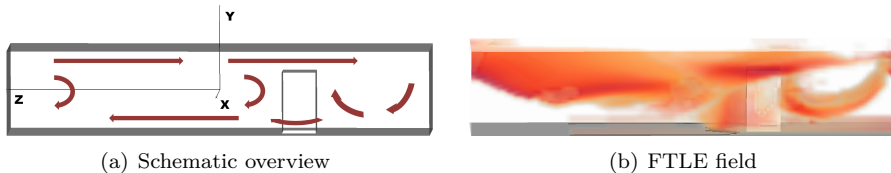
Figure 4.1: (a) Schematic overview over the flow domain, z being the streamwise direction. (b) A FTLE field of a simulation of a bursting dam. The FTLE values lower a certain threshold are rendered transparently. We see that we can identify expected structures around the obstacle. The upper rear part of the flow domain shows large regions with high FTLE values, presumably induced by shearing.
