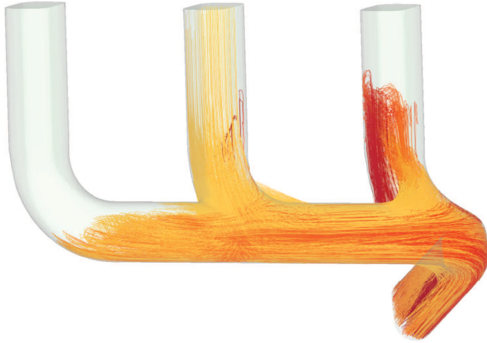
Figure 4.5: Path lines in a exhaust manifold. All displayed path lines are seeded in the vicinity of the middle inlet pipe. The color encodes integration time (yellow to red). Particles moving away from the outlet (lower right corner) first are associated with back pressure.
