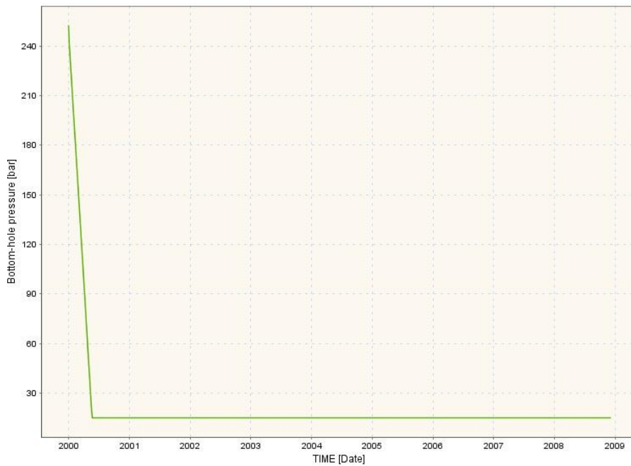
Figure 4.24 Bottom hole pressure on the oil producer well. It presents the same anomaly than the previous producer well in the first simulation, the BHP drops until 15 bars and remains the same during all the simulation time.
