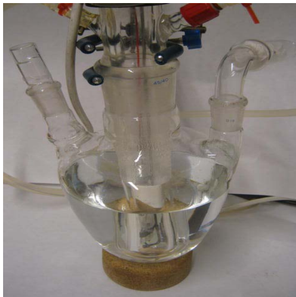
Figure 4.4: Photochemical reaction set-up
