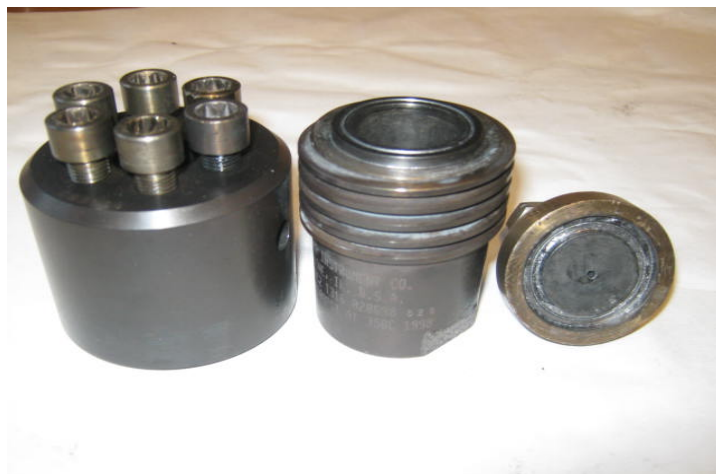
Figure 4.1: Disassembled reactor (20 ml) for pyrolysis oxidation reactions
