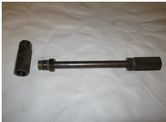
Figure 4.2: Disassembled reactor (5 ml) for peroxide oxidation reactions
