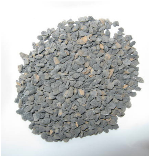
Figure 4.3: Leca particles of 1.5 - 2.5 mm size range
