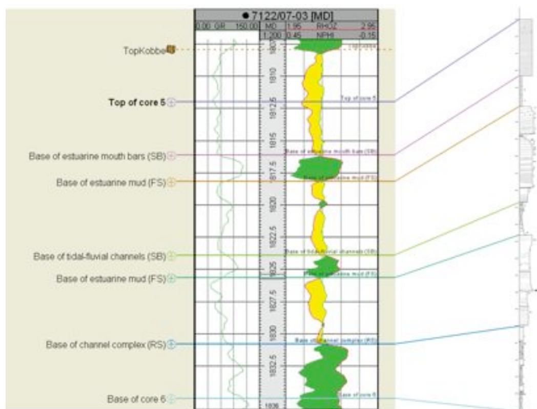
Figure 54 - Well 7122/7-3. Data collected from wireline logs and the interpreted core. GR = Gamma ray, RHOZ = Density, NPHI = Neutron porosity. Log not to scale
