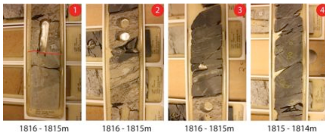
Figure 41 – (1) Sequence boundary. (2) Poorly sorted conglomerate with organic material. (3) Lenticular bedding. (4) Bioturbation (yellow circles)
