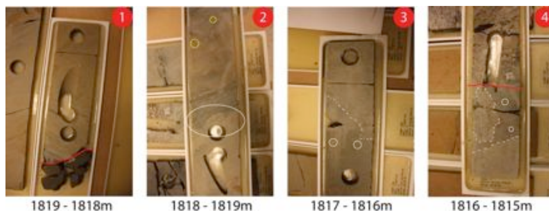
Figure 40 - (1) Erosional boundary generating a sequence boundary. (2) Bioturbation and limestone concretion. (3) Limestone concretion. (4) Erosional boundary between FA1 and FA2
