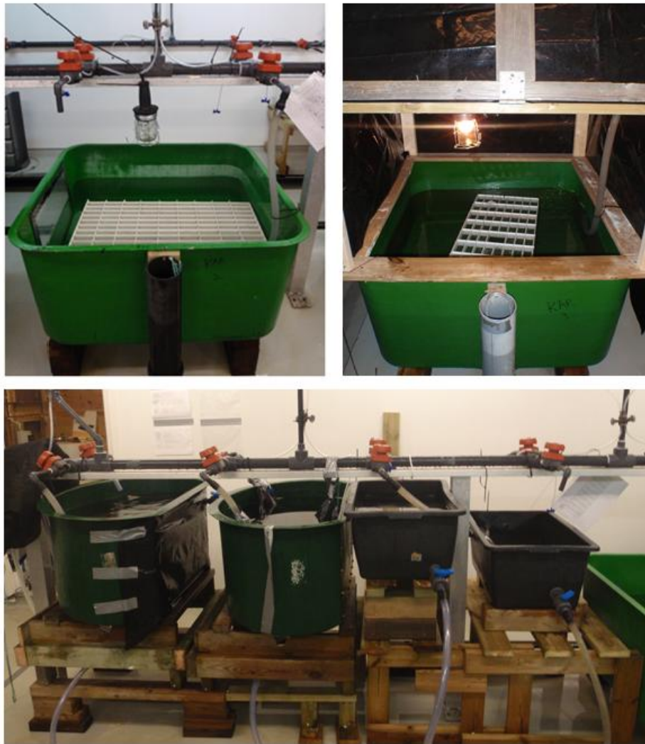
Figure 3: Tank setup (flow through system). Upper: Summer (left) and Winter (right) lobster tanks. Inflow regulated with globe valves and volume fixed to 300 l through a lateral standpipe. Lights controlled by automatic timers. Lower: Predator tanks and collection tank for predator water. From the left: Elevated tanks for cod, wrasse and crab. Water was descending by gravity to the collection tank, and further into lobster treatment tanks (see also Fig. 2) (Photo: H. Trengereid).
