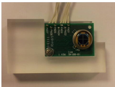
Quadrant cell detector mounted on bracket
