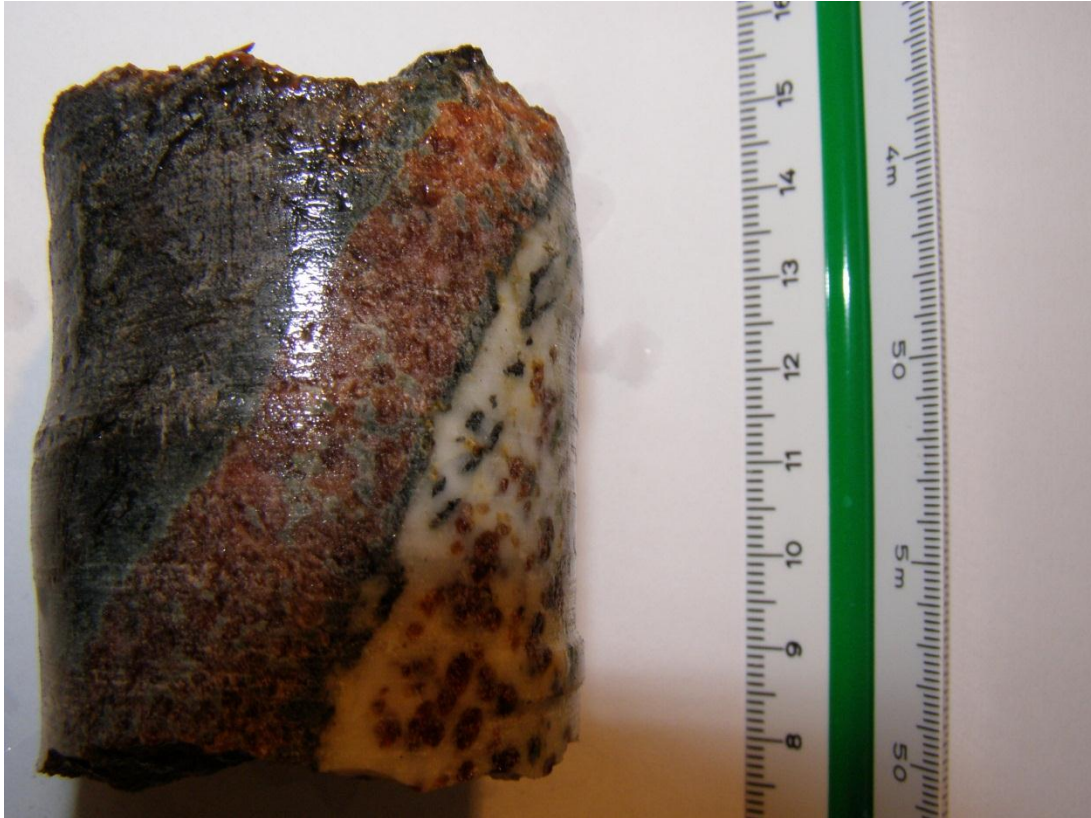
Figure 20: A 7 cm long drilled core from the field area. The sample represents a cut through a corona texture.
