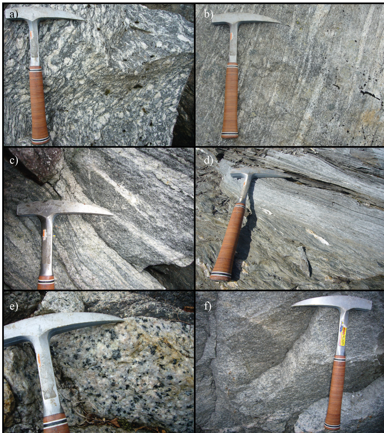
Fig. 14. A selection of the sampled lithologies: a) Augen gneiss with large (~5 cm) feldspar porphyroclasts, sampled on Osafjellet (sample no. KJ-26); b) Stromatic migmatite from the southeastern flank of Onen near Kjeavatnet (KJ-19); c) Strongly foliated biotite gneiss from Osa (KJ-31); d) Quartzitic phyllite with quartz segregations, sampled close to the summit of Nipahøgdi (KJ-24); e) Coarse-grained Eidfjord Granite from Simadalen (KJ-23); f) Massive, medium-grained granite from Bruravik (KJ-27).
