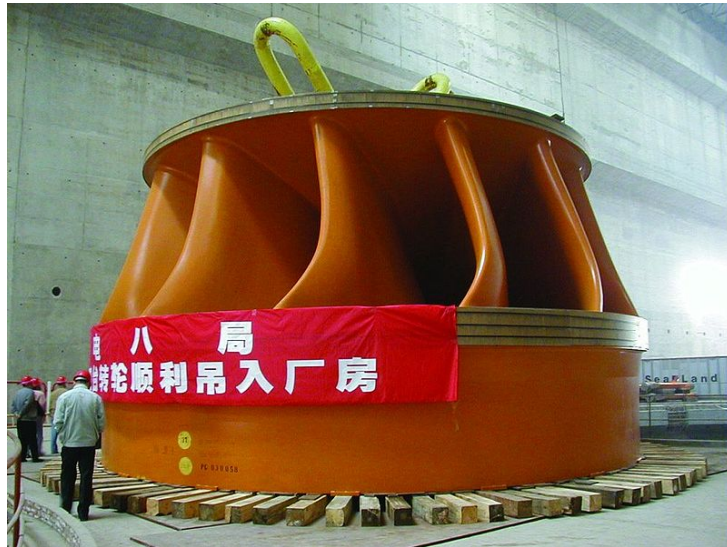
Figure 2.2: Voidth-Siemens Francis runner used in the Three Gorges plant. [133]
