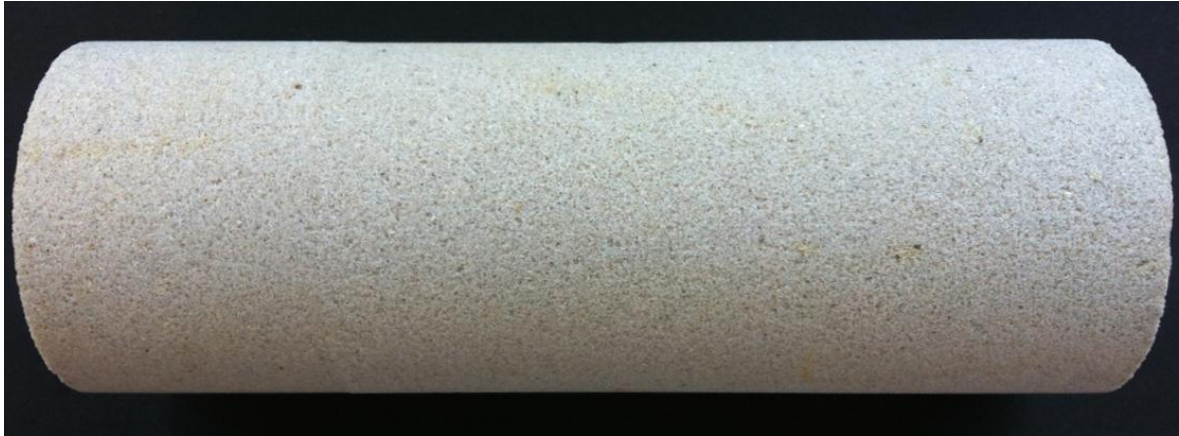
Figure 3.2.2 – Whole Bentheim sandstone core, cut into approximately 5 cm diameter and 14 cm length
