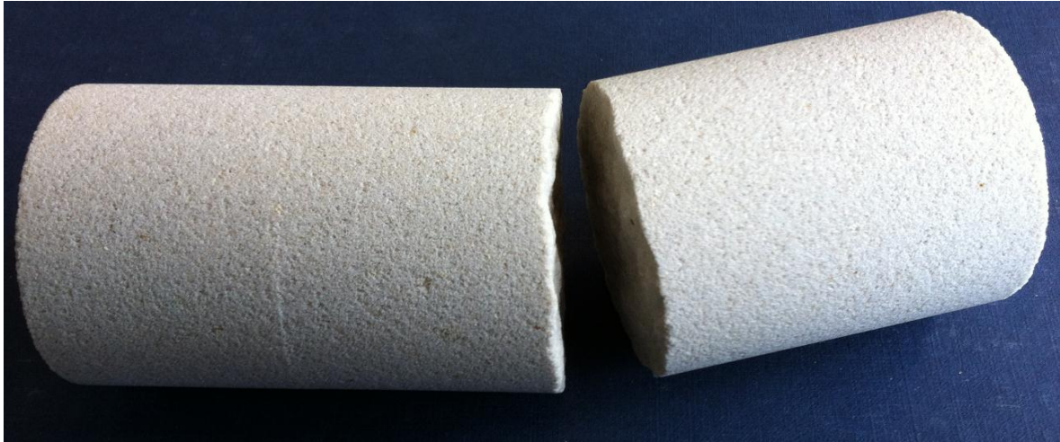
Figure 4.2.7 – Broken core in DEP5. Local differential pressures due to hydrate plugging offers a plausible explanation for the fracture
