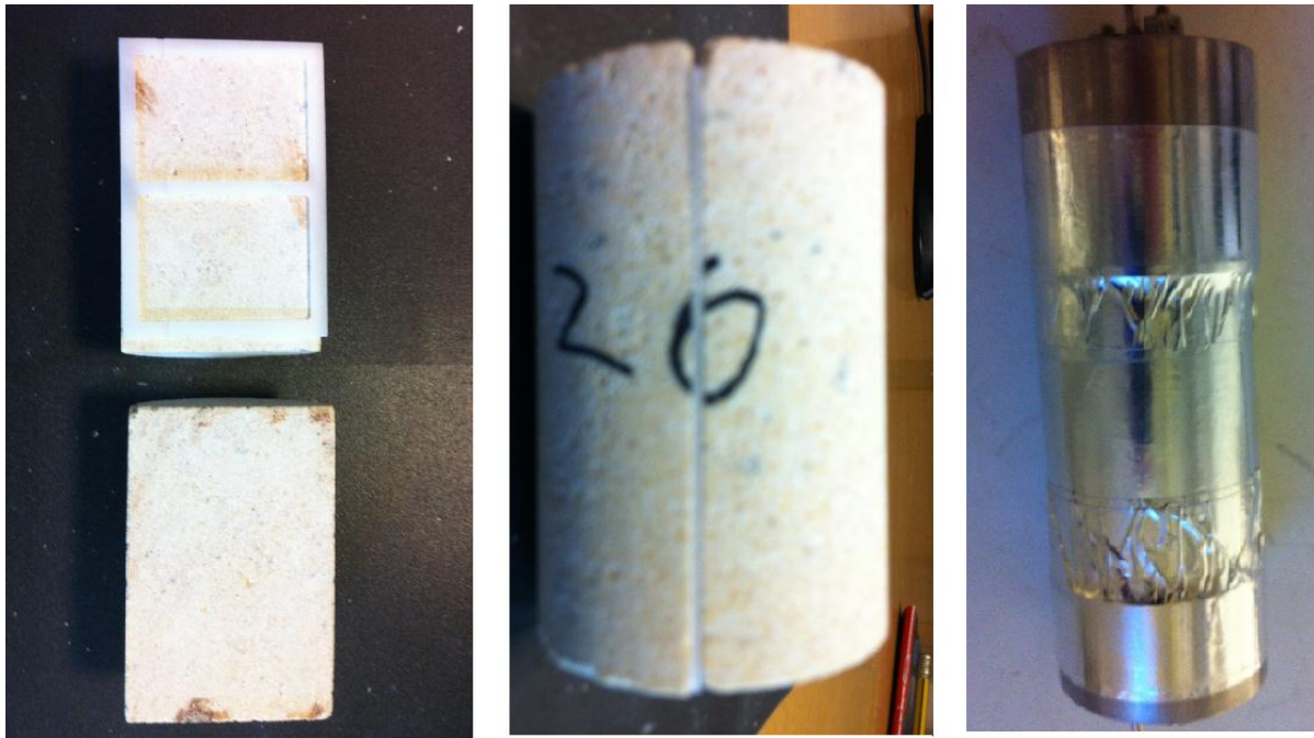
Figure 24: Pictures of a fractured core with spacer. The third picture is the core and the end-points wrapped in aluminum.
