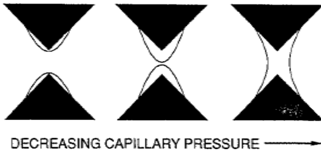
Figure 15: Schematics of snap-off in a pore-throat. (Rossen, 1996)
