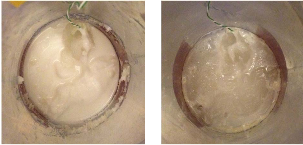
Figure 5.10: (a) Cyclopentane hydrate after removing the mixer. (b) Pure Cyclopentane hydrate at the end of the experiment.
