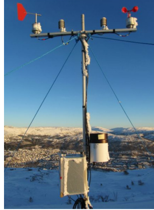
Figure 5.1: AWS at Mount Løvstakken. From the left: Sensor for wind direction, temperature, relative humidity and wind speed. Gust is measured by the same sensor as wind speed. The data logger, the DSU and the batteries are inside the box. HOBO rain gauge is mounted above the box at 110 cm above ground (black and white cylinder). The four ropes are attached to poles of either wood or steel in the ground. An early stage of icing at the sensors can be seen in the picture.
