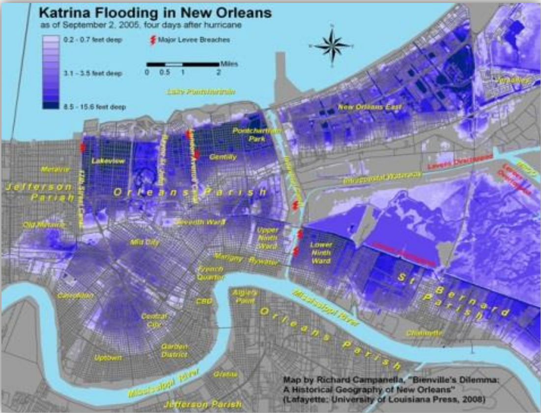
Figure 5. - Map of the floodwaters, indicating water depth four days after flooding (Campanella 2008).
