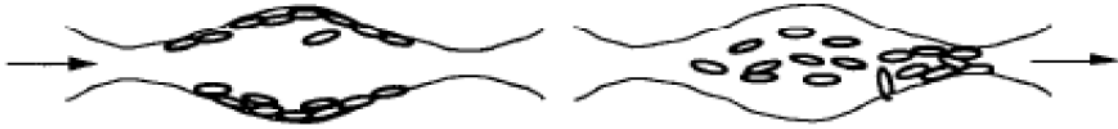
Figure 3.2: Reduced salinity of invading brine causes release of clay fines from pore walls that results in blocking of pore throat entry, a process called log-jamming. [5]
