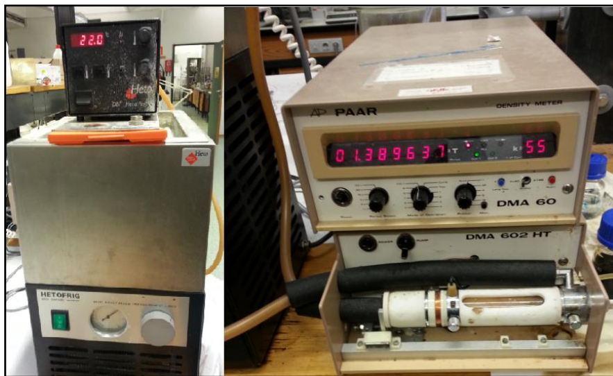
Figure 6.11: Hetofrig water bath connected to Anton Paar Density meter
