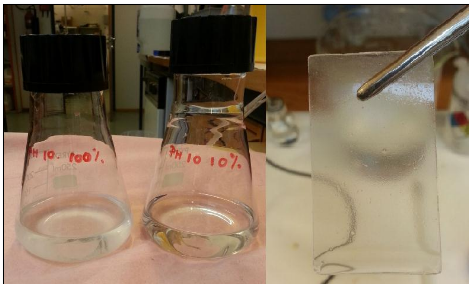
Figure 7.6: Illustration of the precipitated material in pH 10, 100% SSW, compared with the almost blank pH 10, 10% SSW, and a glass slide covered with the precipitated material.
