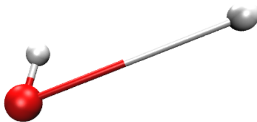
FIGURE 7.19: Abnormal bond stretching in water caused by scaling the repulsive part of the potential faster than the electrostatic part. The length of the stretched bond is \sim 6 Å, while the equilibrium O-H bond length in SPC water is 1 Å.
