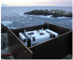
Figure 1. The WindCube LIDAR (Light Detection And Ranging) device at Storholmen. The photo is provided by Vestavind Offshore.
