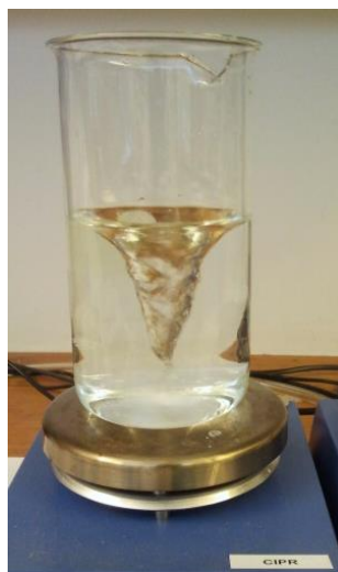
Figure 3.2 The vortex created by magnetic stirring.
