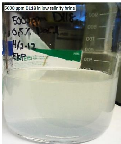
Figure 3.4 A homogenous polymer stock solution after mixing overnight (5000ppm solution of D118 in low salinity brine).
