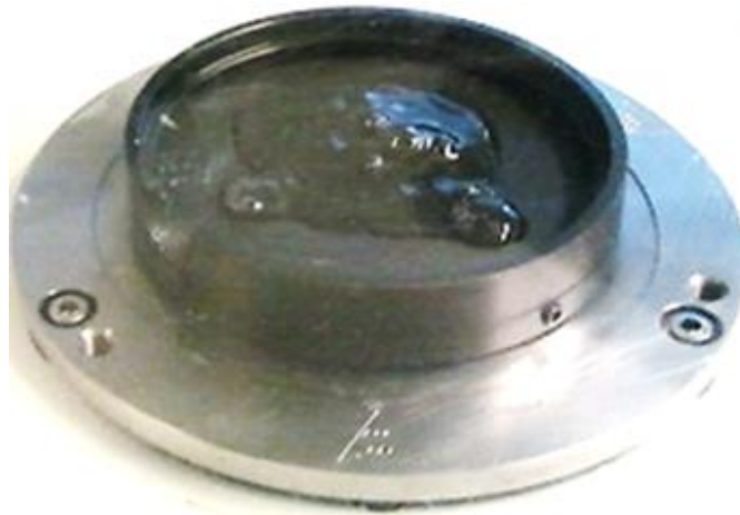
Figure 3.12 Difficulties when sampling the extremely viscous 5000ppm solution of B192 in the high salinity brine.
