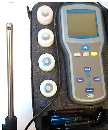
Figure 3.15 the pH- meter from Hach- Lange with ISFET and glass pH probe.
