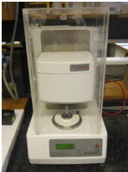
Figure 3.10 MCR300 Rheometer by Anton Paar covered by a Plexiglas.
