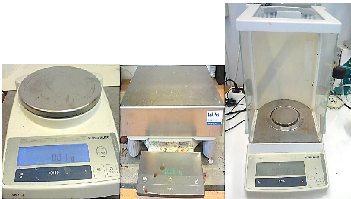
Figure 3.18 Weighing scales. Left: PB 3002S, middle: SG 16001g, right: AB204-S.
