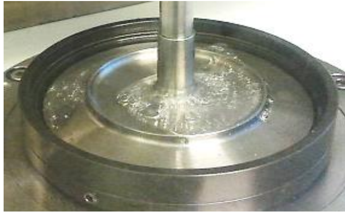
Figure 3.14 Unstable measurements at high shear rates due to Weissenberg effect or phase transition of concentrated polymer solutions. 5000ppm solution of C319 in low salinity brine is photographed.
