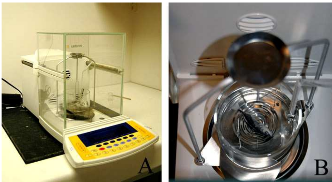
FIG 8A. Sartorius Genius Series ME5 with YDK 01; B. YDK 01 setup while measuring a stickleback
