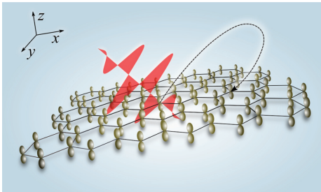
FIG. 1. (Color online) Artist's impression of graphene exposed to a linearly polarized laser pulse. The graphene layer is modeled by hydrogenic p_z orbitals distributed on a honeycomb lattice in the xy plane, and the polarization vector of the laser pulse is tilted with respect to the z axis. The trajectory illustrates the situation in which the ionized electron recombines with another atom in the lattice.
