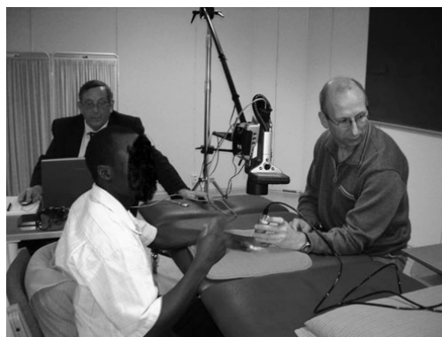
FIG. 1. Laboratory setup. Thermographic camera placed approximately 25 cm over the subject's hand, with the participant sitting at a table with both hands on a towel.
