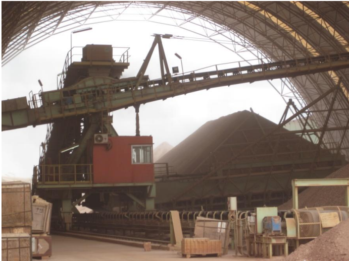
Figure 6: An automated machine (stacker) in the new production line had replaced the crane for feeding raw materials onto the conveyor belt (Photo by Tungu)
