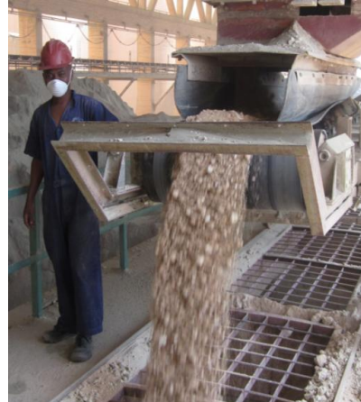
Figure 4: A crusher attendant observing flow of raw materials on the old crusher conveyor belt (Photo by Tungu)
