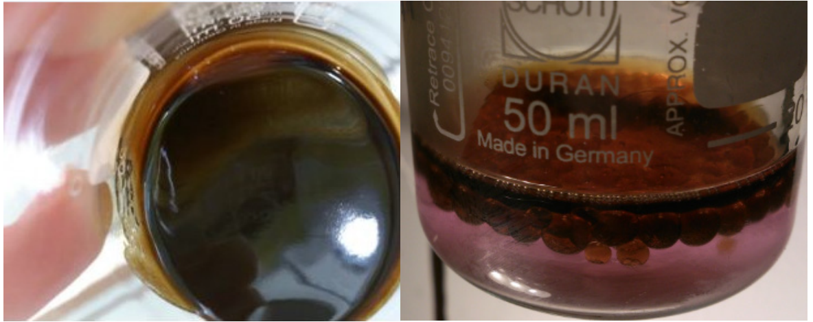
FIGURE 2.2: Example pictures of emulsion states taken during laboratory experiments by the author. Left: water-in-oil emulsion, right: oil-in-water emulsion.
