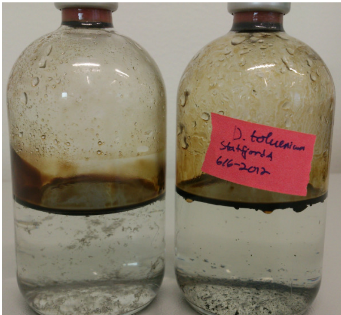
FIGURE 3.14: Pure medium with non-degraded Statfjord A (left) and biodegraded Statfjord A and medium containing D. toluenicum cultivated on crude oil for 10 months (right.)
