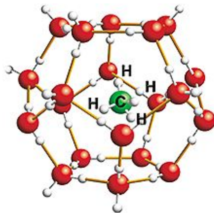
FIGURE 1.1: A simplified structure I representation of a methane hydrate, adapted from Schlumberger.[14]
