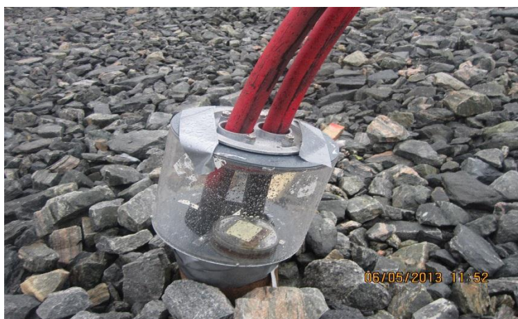
Figure 6.1 Coal box inside a closed box on the top of borehole in order to absorb radon gas in area3.
