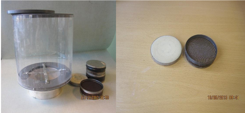
Figure 3.2: Radon test equipment (coal box).
