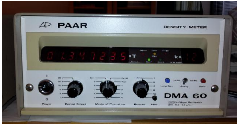
Anton Paar DMA60 densitometer.
