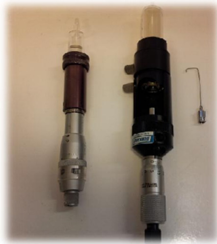
Figure 5.5 Micrometer syringe from Burkard (to the right) used to measure the interfacial tension. The inverted needle is also shown.
