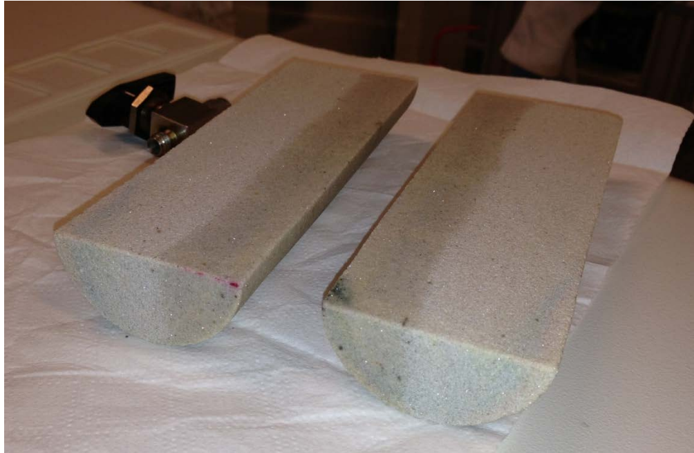
Figure 6.43: Image of the core after ended experiment. The oil is displaced from the top of the core. Remaining oil in the bottom parts of the core was observed and supported the prediction of gravity override of CO 2 in the fracture during the injection test.
