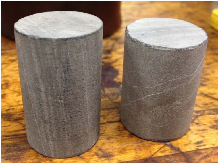
Figure 5.2: Reservoir shale cores containing light crude oil.
