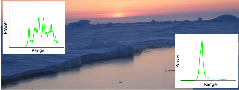
Figure 1.4: Typical waveform shapes over sea ice and leads from the radar altimeter SIRAL on-board CryoSat-2. The return signal from leads is specular while over sea ice the echo signal is diffuse.
