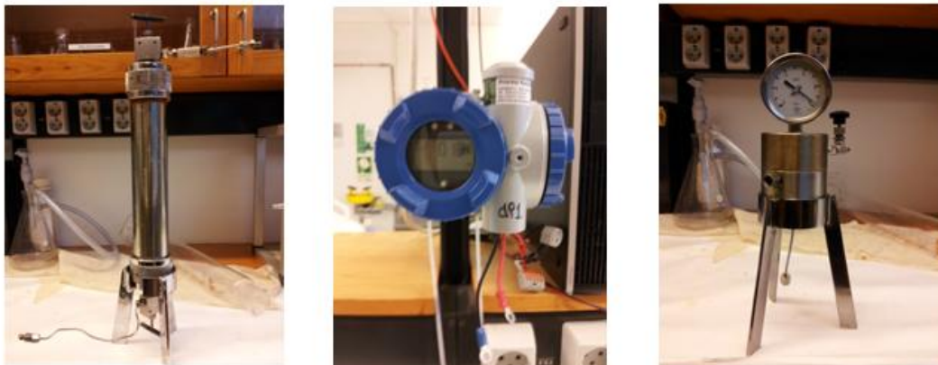
Fig.7.7: Left picture: Piston cylinder. Middle picture: Fuji electric FCX-FKC differential pressure transducer. Right picture: Back pressure regulator.
