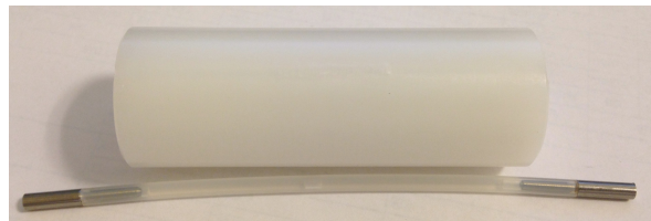
Figure 3.5: The mouse-like phantom. The clear flexible tubing can be inserted into a cylindrical hole, 10 mm from the central axis of the phantom.
