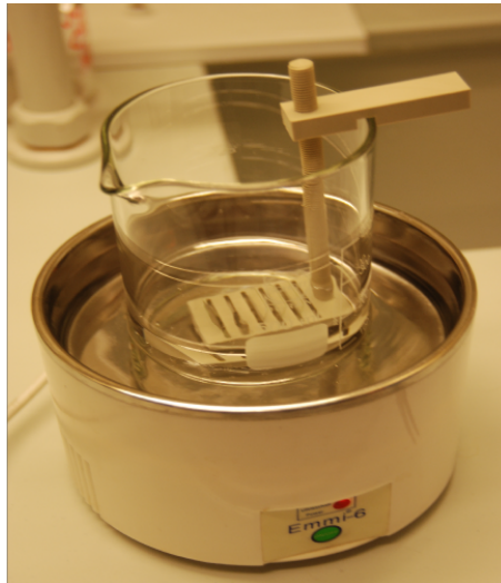
Figure 5.1: Image of the ultrasonic bath used for substrate cleaning. Note that the sample holder used in the cleaning process is depicted.
