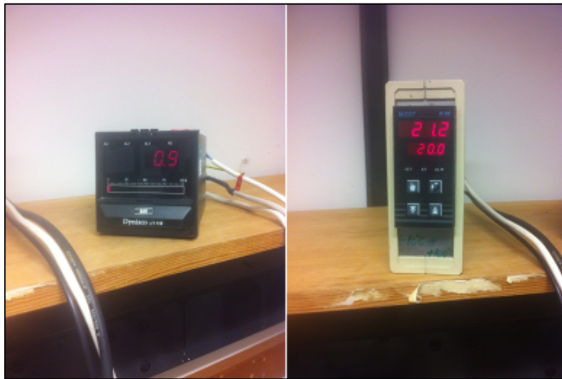
Figure 3.6: The Dynisco \mu PR700 pressure indicator to the left, and the West 8100 temperature controller to the right.
