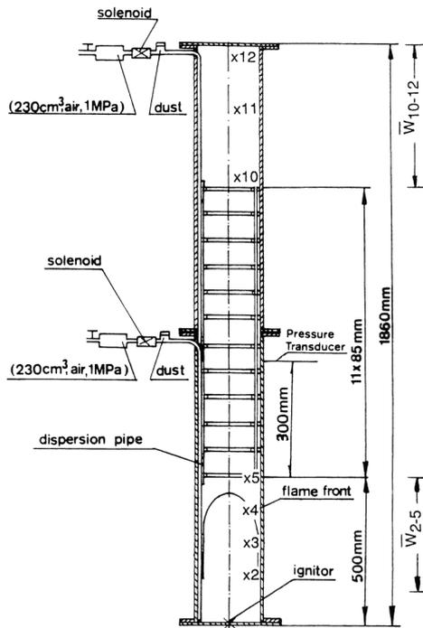
**Figure 1** Schematic diagram of apparatus for explosion tests, from Pu et al. (1988). The closed tube is 0.19 meters in diameter and 1.86 meters long. It is filled with ring-shaped obstacles, and equipped with a piezoelectric pressure transducer and ionisation probes for measuring flame arrival. The ignition source was 0.6 grams of black powder, with total energy release about 1.75 kJ in 25 ms.
