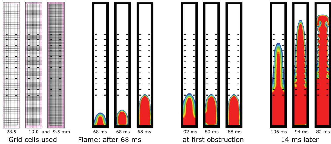
**Figure 5** Vertical cross-section of simulated pipe, illustrating grid cells and simulated flame development for various grids during a cornstarch-air explosion. Flames are plotted as mass fraction of combustion products at various time-steps: after 68 ms, when the flames reaches the first obstruction, and 14 ms after the flames reached the first obstruction. The modelled cornstarch had a  $K_{St}$  value of about 150 bar m/s.
