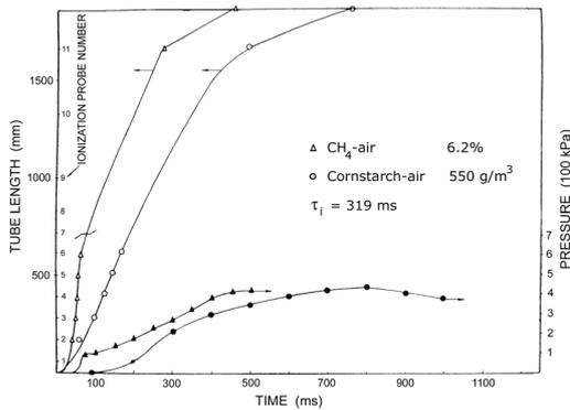
**Figure 2** Pressure rise and location of flame front as functions of time in 1.86 meter closed tube for mixtures of 6.2 % methane in air and 550 g/m<sup>3</sup> cornstarch in air (from Pu, 1988).
