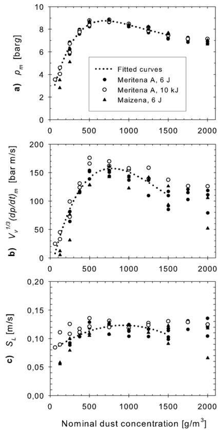
**Figure 3** Experimental results for two types of dried cornstarch: **a)** corrected explosion pressure, **b)** size-normalized rate of pressure rise (maximum value corresponding to a  $K_{st}$ -value of about 150 bar m/s), and **c)** estimated laminar burning velocities.
