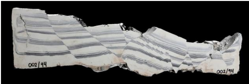
Figure 4.7: Extensional plaster model from 1994, made by Fossen and Gabrielsen (Picture by Simon Buckley).
