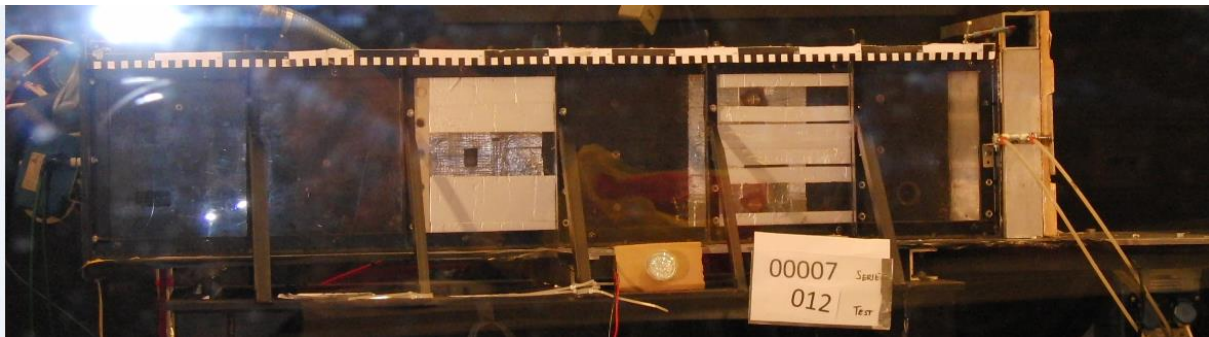
Figure 1-5: The 0.3x0.3x1.5 m MOGELEG channel with transparent plastic front side. Closed end to the left and open end to the right..
