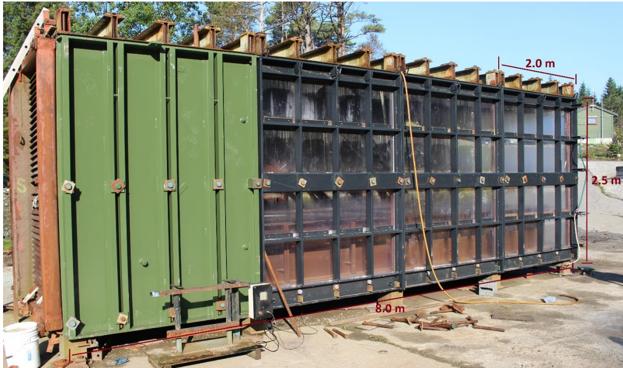
Figure 3-14: The 50m 3 module used for large-scale testing.
