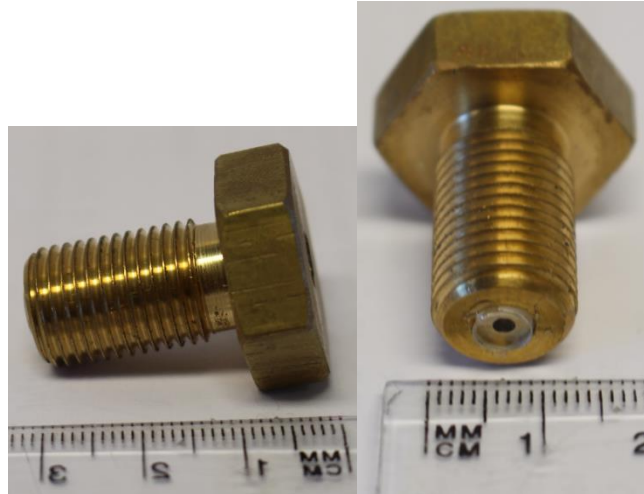
Figure 3-5: A line of sight detector without fitted photodiode.
