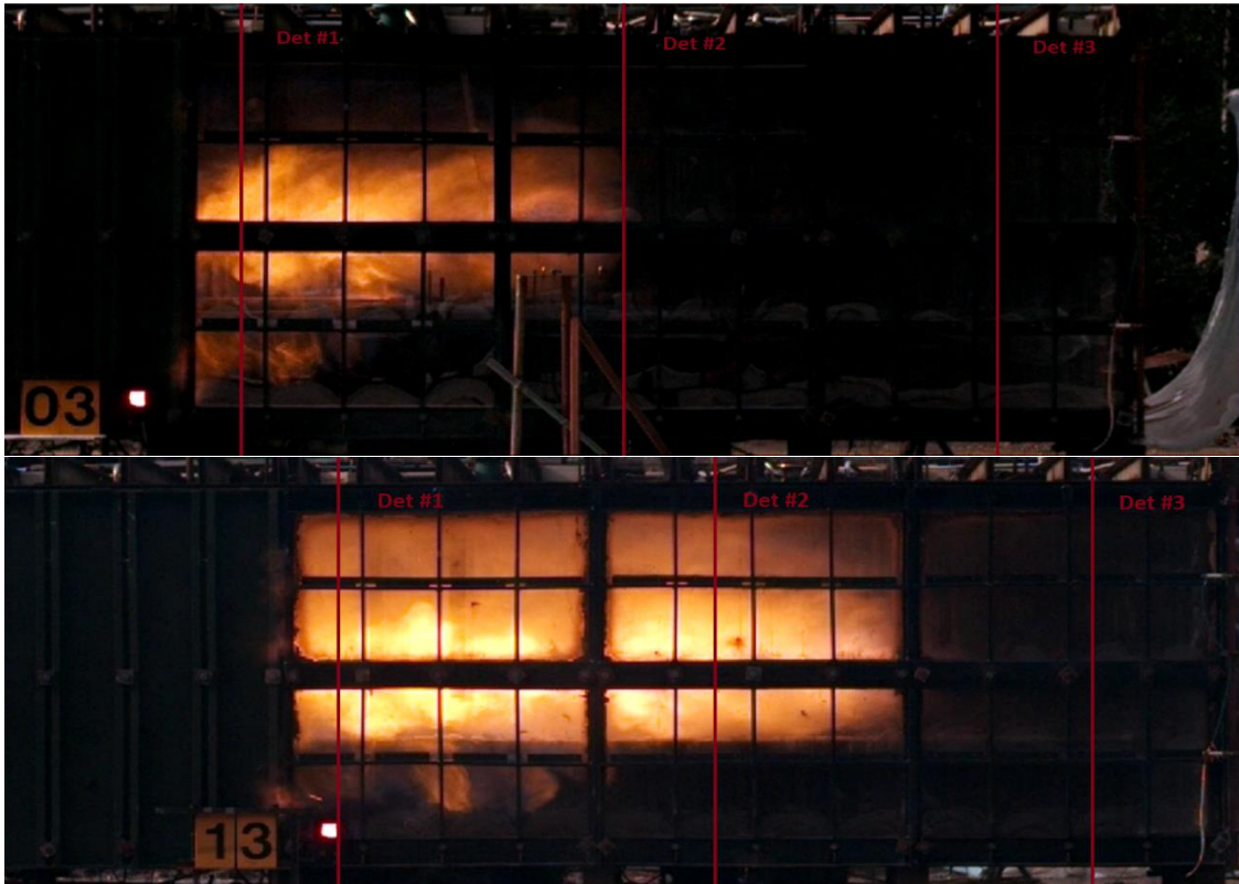
Figure 4-31: Comparison of measured flame front positions by detector #3 during tests 003 and 013.
