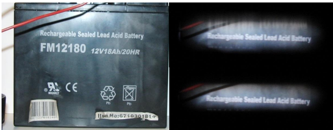
Figure 4-16: Left: Reference picture, top right: slit before roughening with sandpaper, bottom right: slit after roughening with sandpaper.
