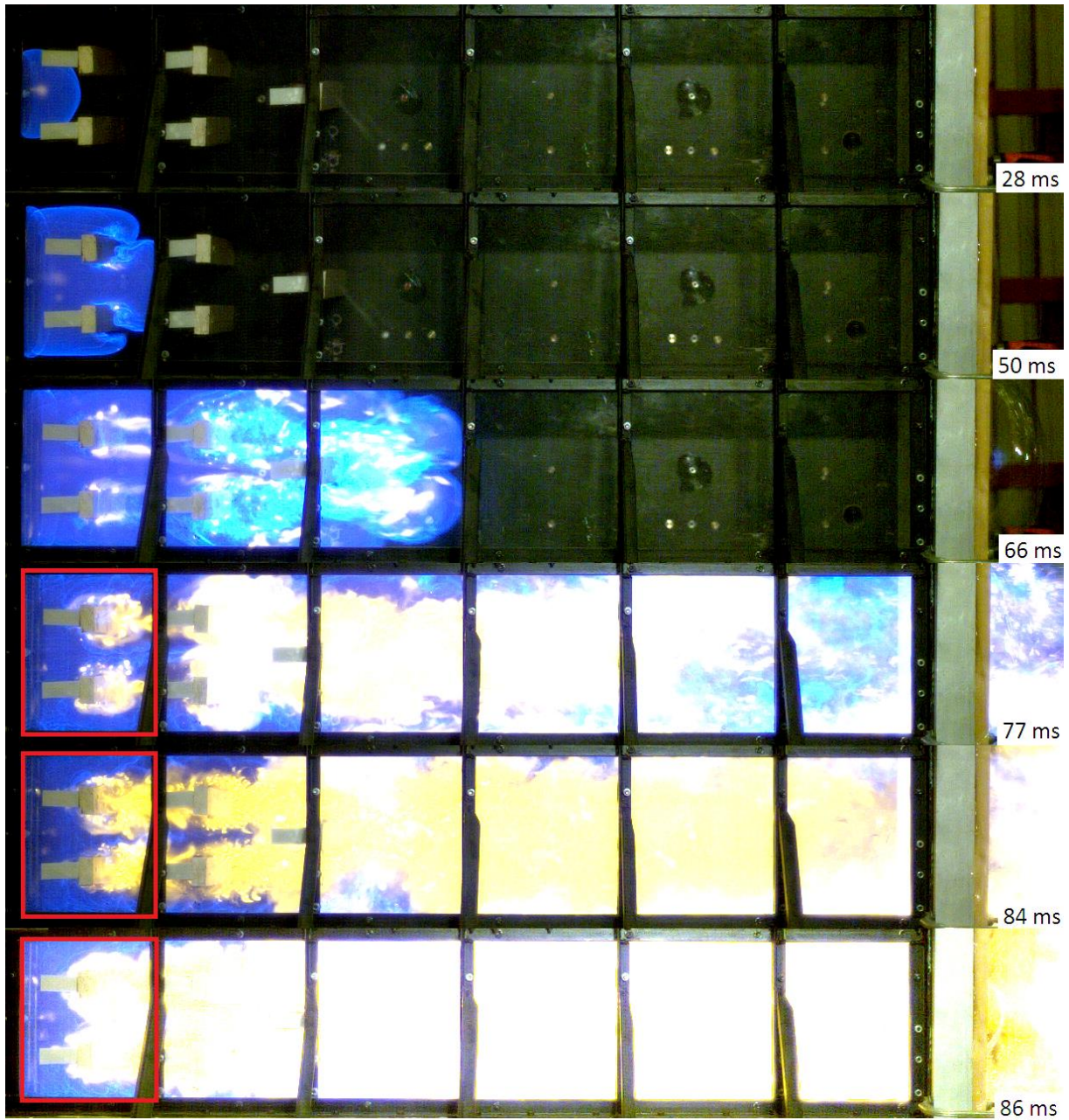
Figure 2-32: Explosion experiment in MOGELEG channel with fuel-air ration equal 1.4[32].
