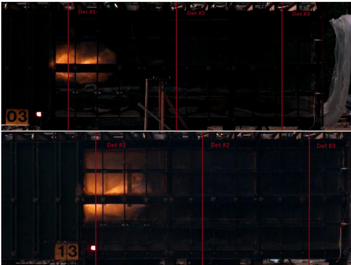
Figure 4-30: Comparison of measured flame front positions by detector #2 during tests 003 and 013.
