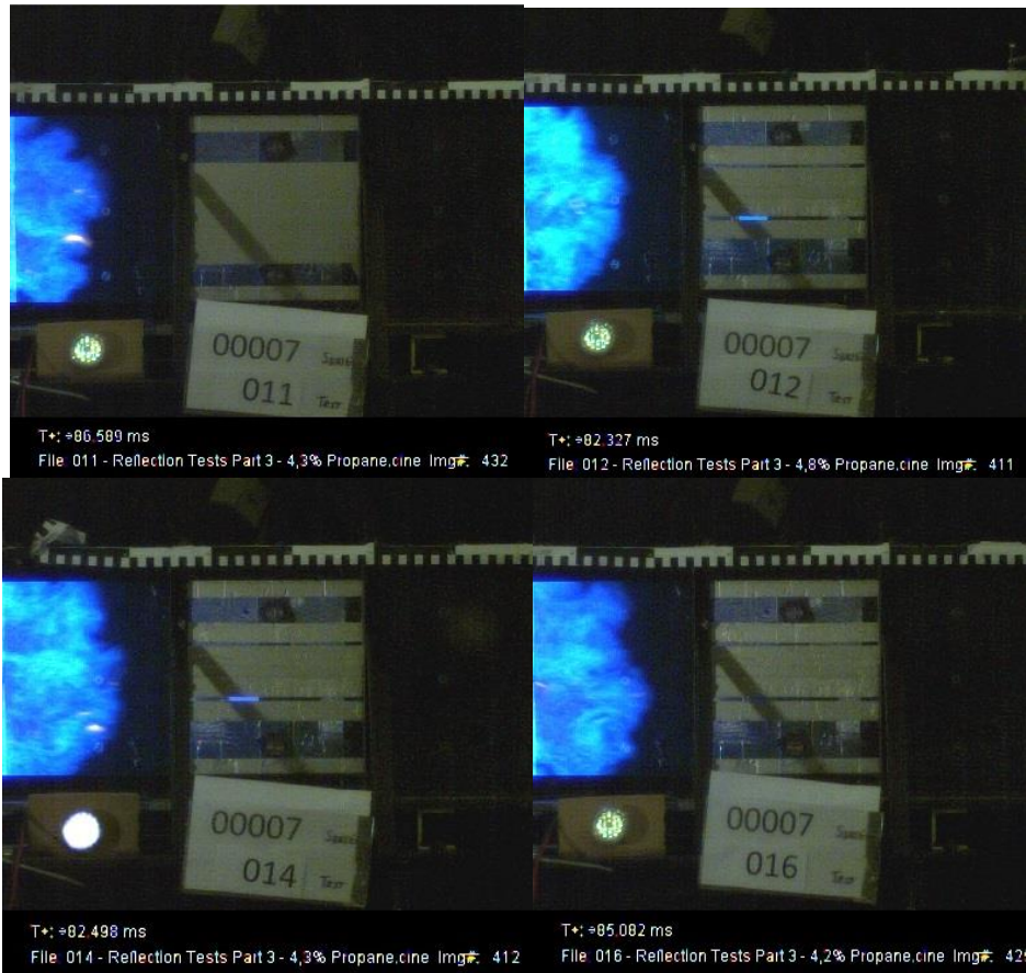
Figure 4-19: Top left: first reflection configuration, top right: Extreme reflection, 4.8% propane. Bottom left: Extreme reflection, 4.3% propane, bottom right: no extreme reflection, 4.2% propane.
