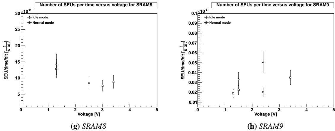
Figure 6.7: Cross section for different voltages at IFE.
