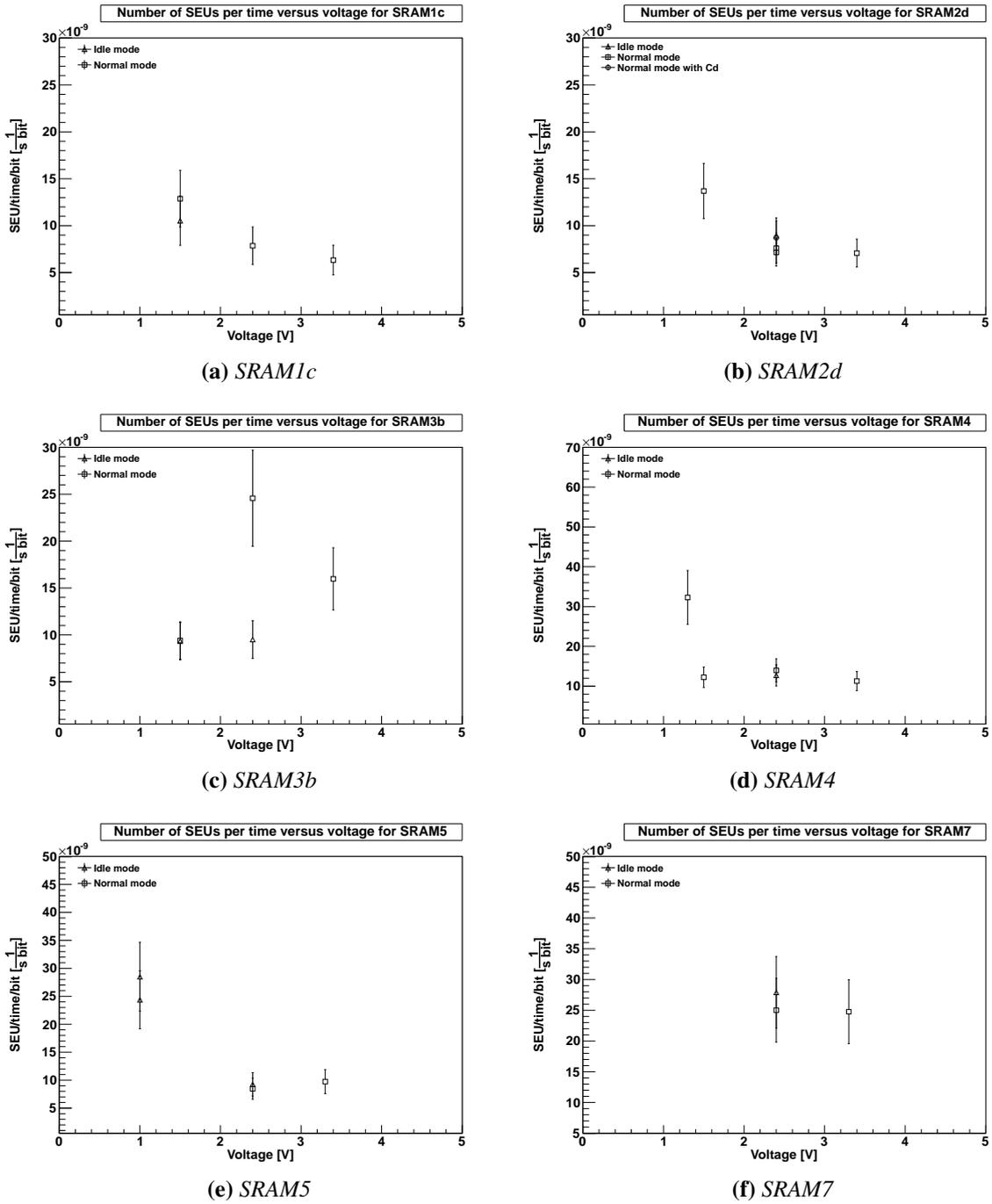
Figure 6.7: Cross section for different voltages at IFE.
