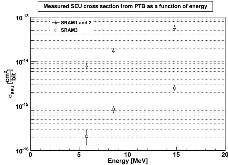
Figure 6.1: Measured SEU cross section as a function of energy.
