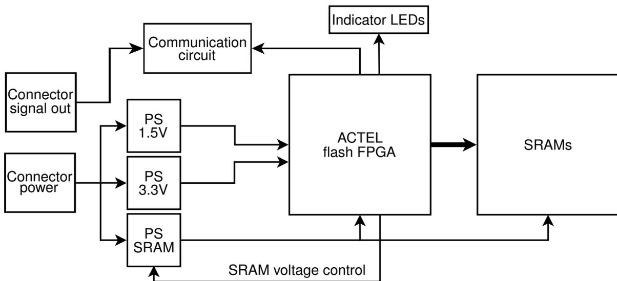
Figure 4.2: Schematic overview of hardware for the detector.
