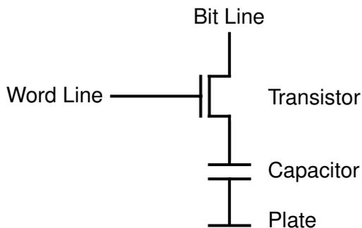
**Figure 3.2:** Schematic drawing of 1T DRAM cell [16].
