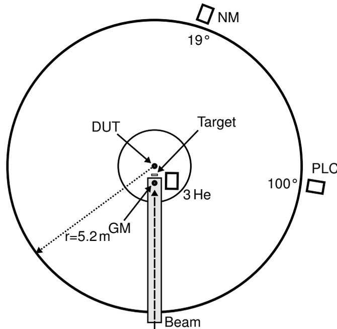
**Figure 5.1:** Schematic setup of the different reference detectors.
