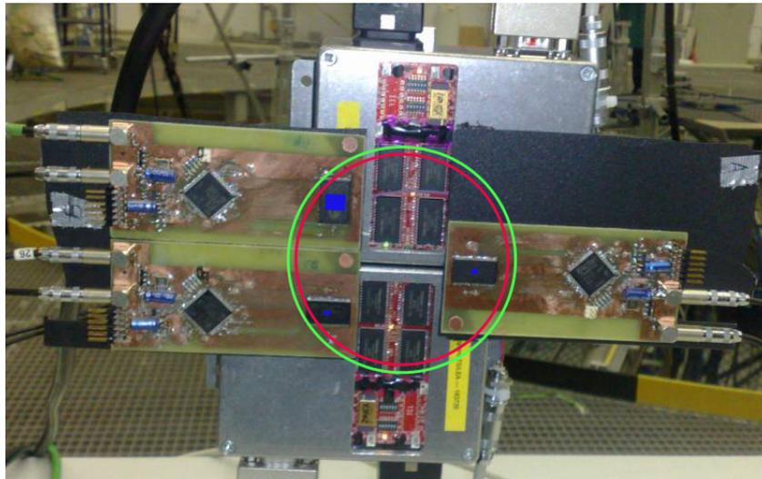
**Figure 5.2:** Photograph of the setup of the SRAMs and RadMon boxes. The green circle indicates the 90 mm diameter, the red circle indicates the 84 mm diameter. The blue squares indicate the size and placement of SRAMs' die. Top left is SRAM2b, bottom left is SRAM1a, right is SRAM1b. SRAM2b was exchanged with SRAM2a when doing the irradiation testing. SRAM2a has a circuit board with a narrower width which makes it come closer to the center of the beam.
