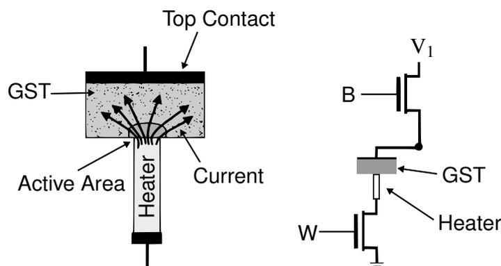
Figure 3.7: Schematic drawing of a PCRAM cell.
