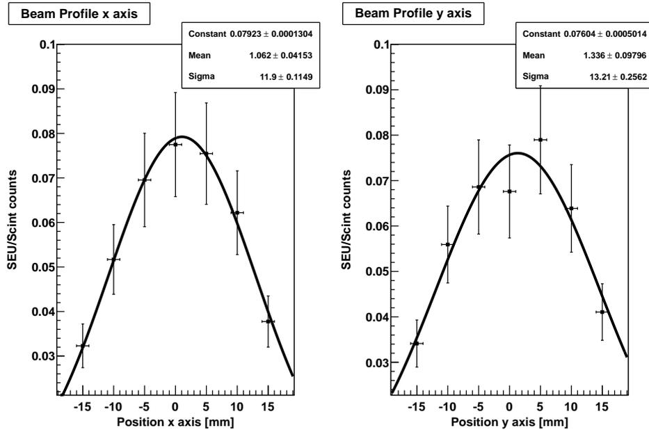
Figure D.3: Beam profile for 9.12.2010. The Gaussian fit was created with ROOT [65].
