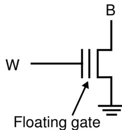
**Figure 3.8:** Schematic drawing of a EEPROM cell.
