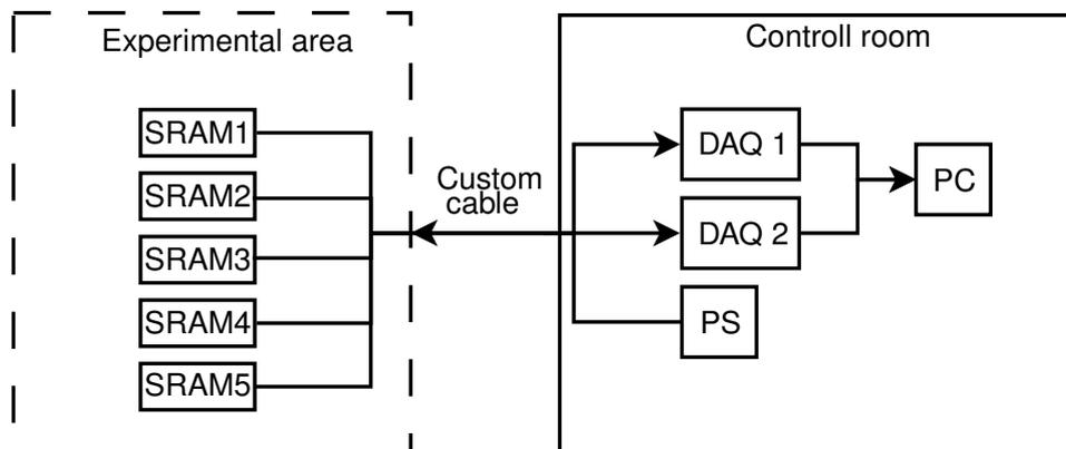
**Figure 5.9:** Schematic setup of the the equipment used at CERF.
