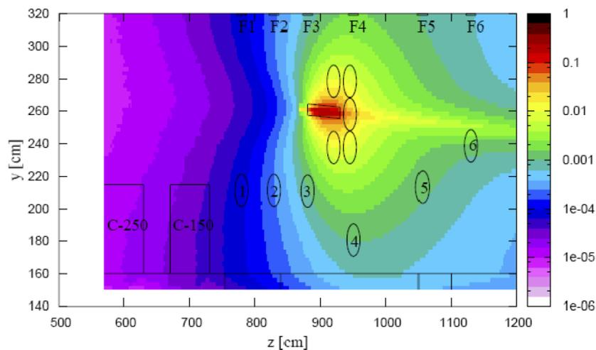
**Figure 5.6:** High Energy Hadrons (HEH) fluence normalized per primary particle on target (p.o.t.) at the different mounting positions [50]. The plot is seen from below.
