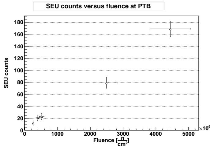
**Figure 6.2:** Number of SEUs as a function of fluence at 8.5 MeV for SRAM1 and 2 combined.
