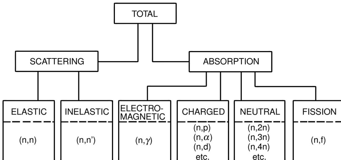
**Figure 2.2:** Overview of different neutron interactions. The letters separated by commas in the parentheses show the incoming and outgoing particle [8].
