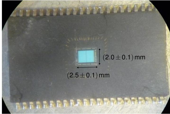
**Figure C.2:** The SRAM used for beam profile measurements. The top has been shaved off after irradiation to expose the die. During irradiation the short end was facing downwards.
