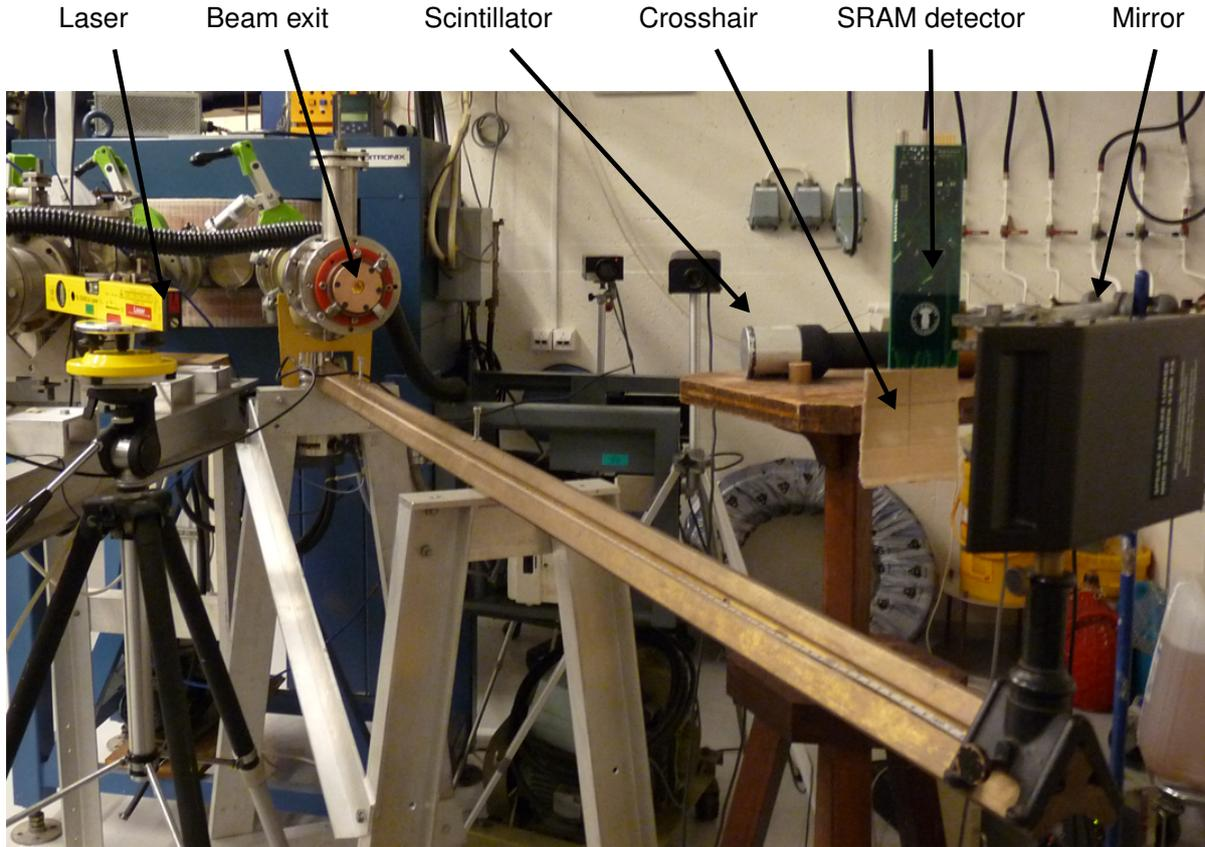
**Figure 5.11:** Overview of setup at OCL.
