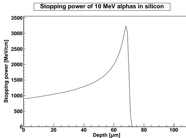
**Figure 2.1:** As an example of the Bragg curve, the stopping power of 10 MeV alphas in  $^{28}\text{Si}$  is shown here as simulated by the SRIM code [7].
