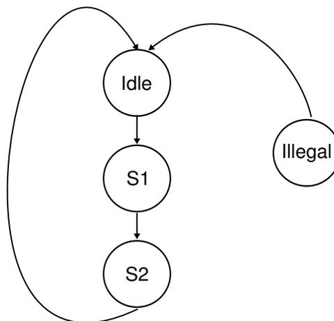
**Figure 4.4:** Illustration of a finite state machine with exit from an illegal state. The next state after the illegal state can also be a special error state which can do some damage control before going to the idle state, but this was not needed in this design.
