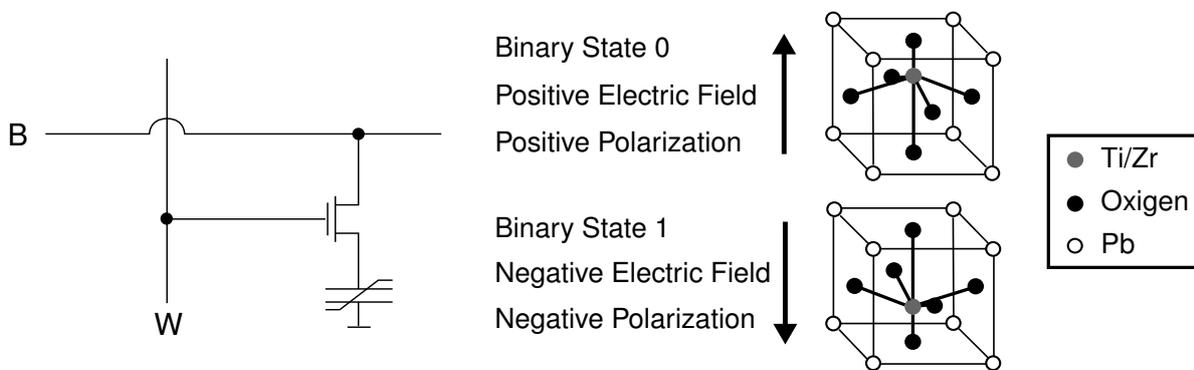
**Figure 3.4:** Schematic drawing of 1T1R FRAM cell [16].
