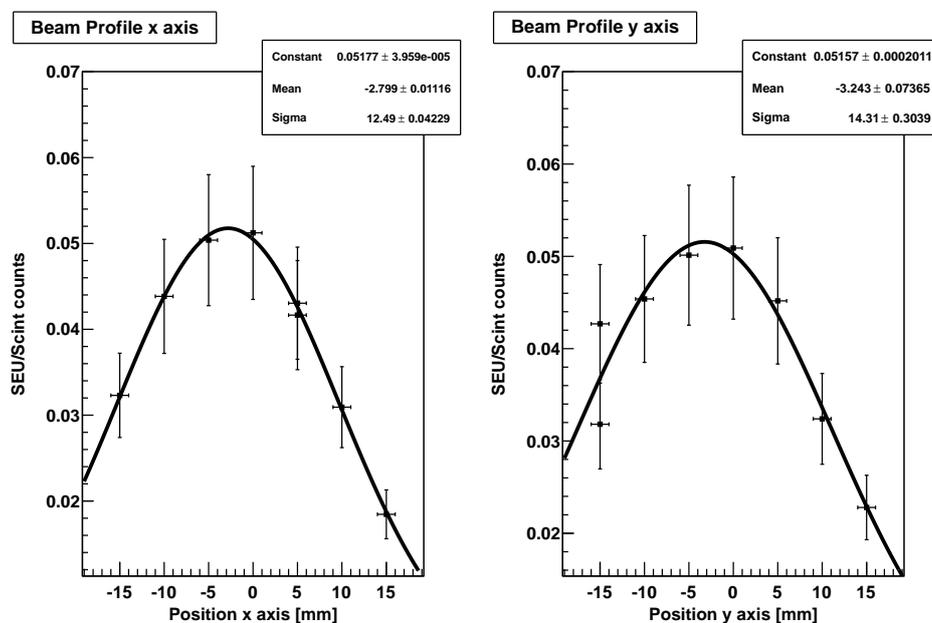
Figure D.2: Beam profile for 8.12.2010. The Gaussian fit was created with ROOT [65].
