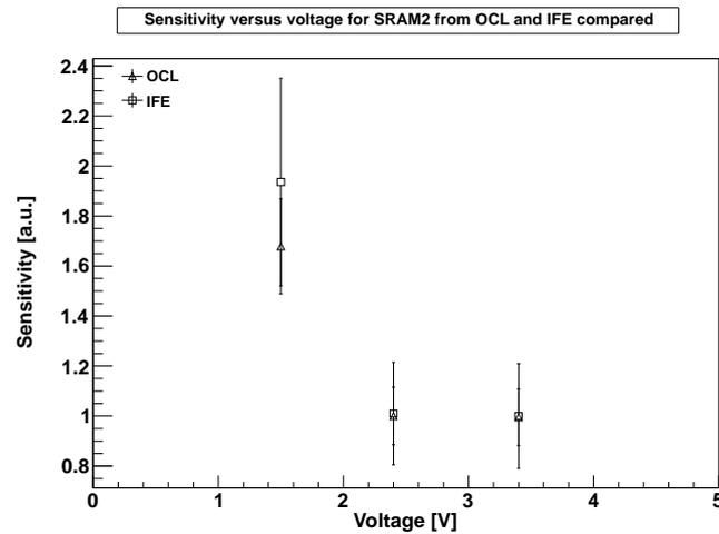
**Figure 7.1:** The voltage dependence of the sensitivity compared between OCL and IFE. The numbers have been normalized to 2.4V and given in Arbitrary Units.
