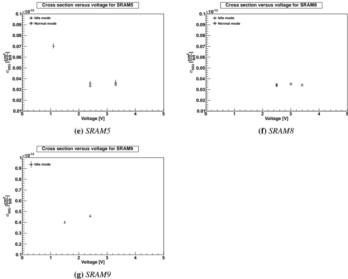
Figure 6.3: Cross section for different voltages at OCL.
