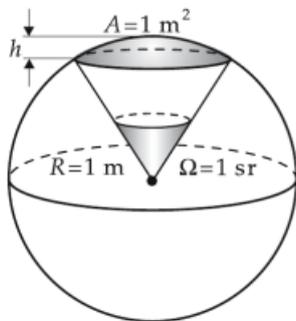
**Figure B.1:** Illustration of the principle of a steradian as a unit of solid angle [64].
