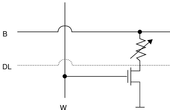
**Figure 3.6:** Schematic drawing of 1T MRAM cell.
