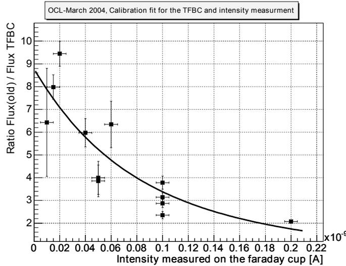
**Figure C.1:** A fit of the ratio between the flux measurement using the Faraday cup and the flux measurement using a Thin Film Breakdown Counter (TFBC) [54].
