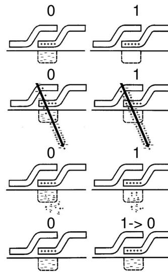
**Figure 3.3:** An alpha particle hitting a DRAM cell can primarily flip a bit from 1 to 0 [23].
