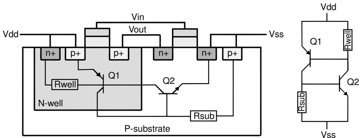
**Figure 2.3:** PNP parasitic structure in an N-well bulk CMOS inverter structure [6].
