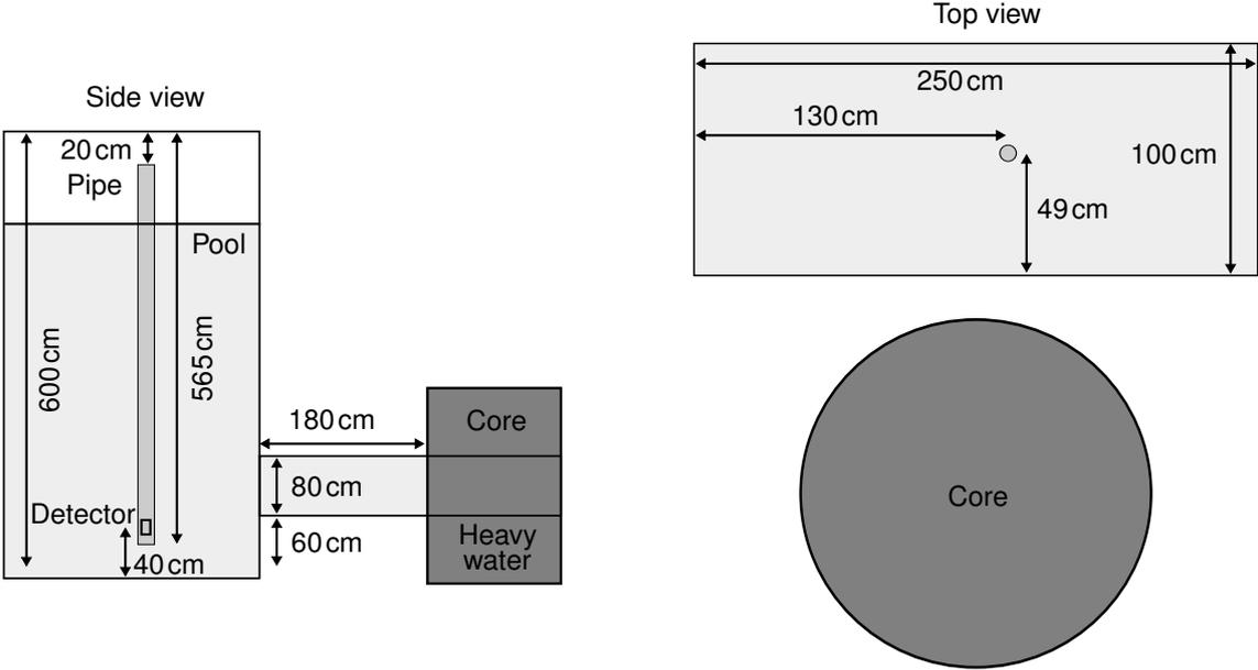
Figure 5.14: Drawing of the placement of the detector in the pool. Not to scale.
