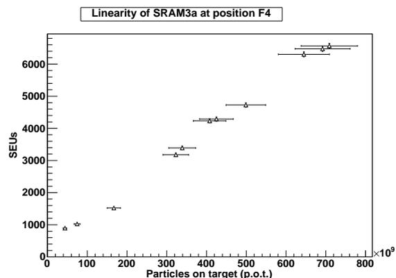
**Figure 6.5:** Linearity of SRAM1b at position F4. **Figure 6.6:** Linearity of SRAM3a at position F4.
