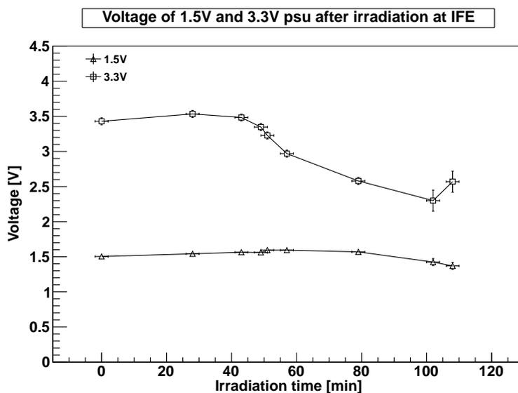
Figure 6.9: 3.3 V and 1.5 V power supply voltage versus irradiation time measured after testing at IFE.
