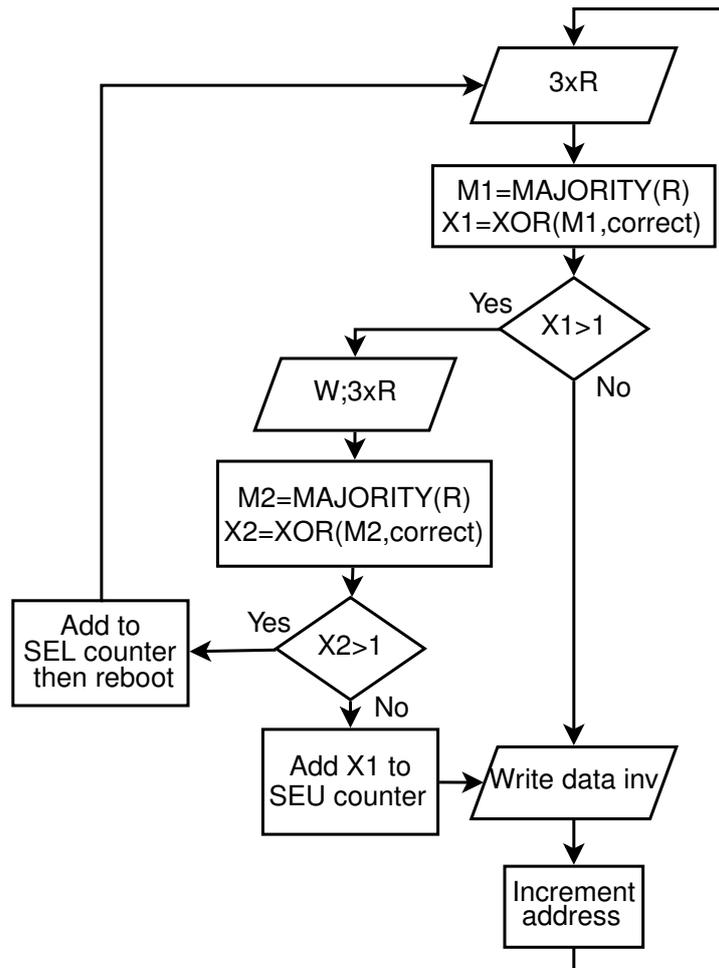
**Figure 4.9:** Flowchart for stuck bit mitigation.
