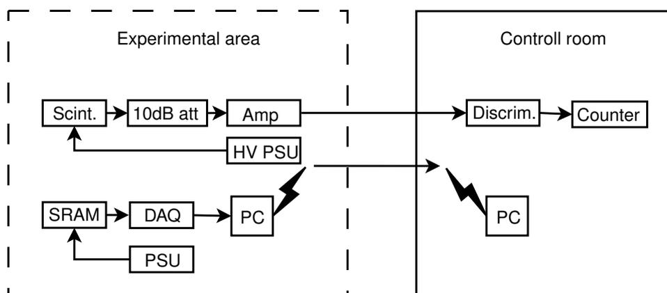
**Figure 5.12:** Schematic setup of the the equipment used at OCL.
