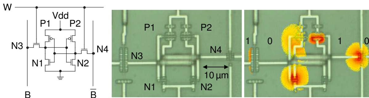
**Figure 3.1:** Image on left shows a standard 6T SRAM cell [16]. Center shows the same cell laid out in a  $0.8\mu\text{m}$  AMS BiCMOS technology, the spacing between transistors are exaggerated for testing purposes. Image on right shows the sensitive areas as mapped by a pulsed laser with energy from  $10\text{pJ}$  to  $1193\text{pJ}$ , darker color indicates higher sensitivity [17].
