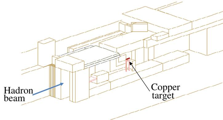
**Figure 5.4:** Layout of the experimental bunker at CERF as modeled in FLUKA [50].
