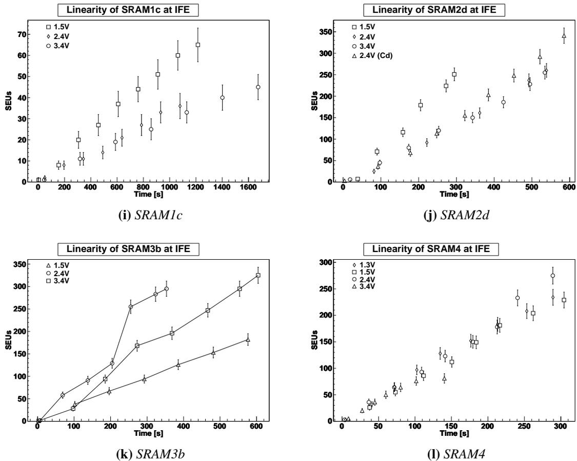
Figure 6.8: Linearity of devices tested at IFE. Lines added for clarity for SRAM3b.
