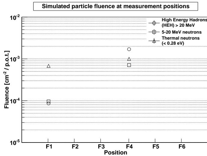
**Figure 5.7:** Simulated fluence for wall positions F1 and F4. Numbers by Ketil Røed [51].
