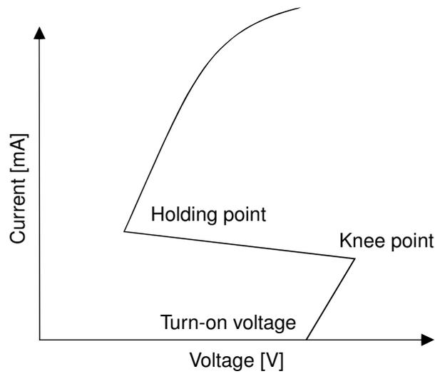
**Figure 2.4:** *The latchup I-V characteristic [15].*
