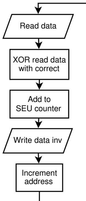
**Figure 4.6:** Simplified flowchart for SEU detection
