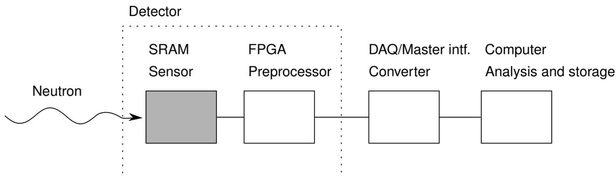
**Figure 4.1:** Overview of a detector system.
