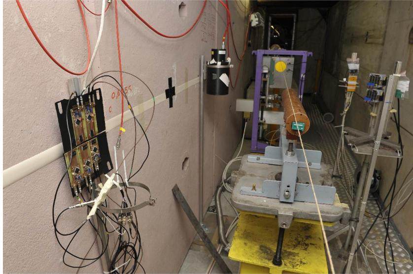
**Figure 5.8:** SRAMs mounted at position F4. Cylinder on right is the copper target, thread indicates direction of incoming particles, horizontal tapelines on wall indicates the height of which the simulated fluence had been calculated.
