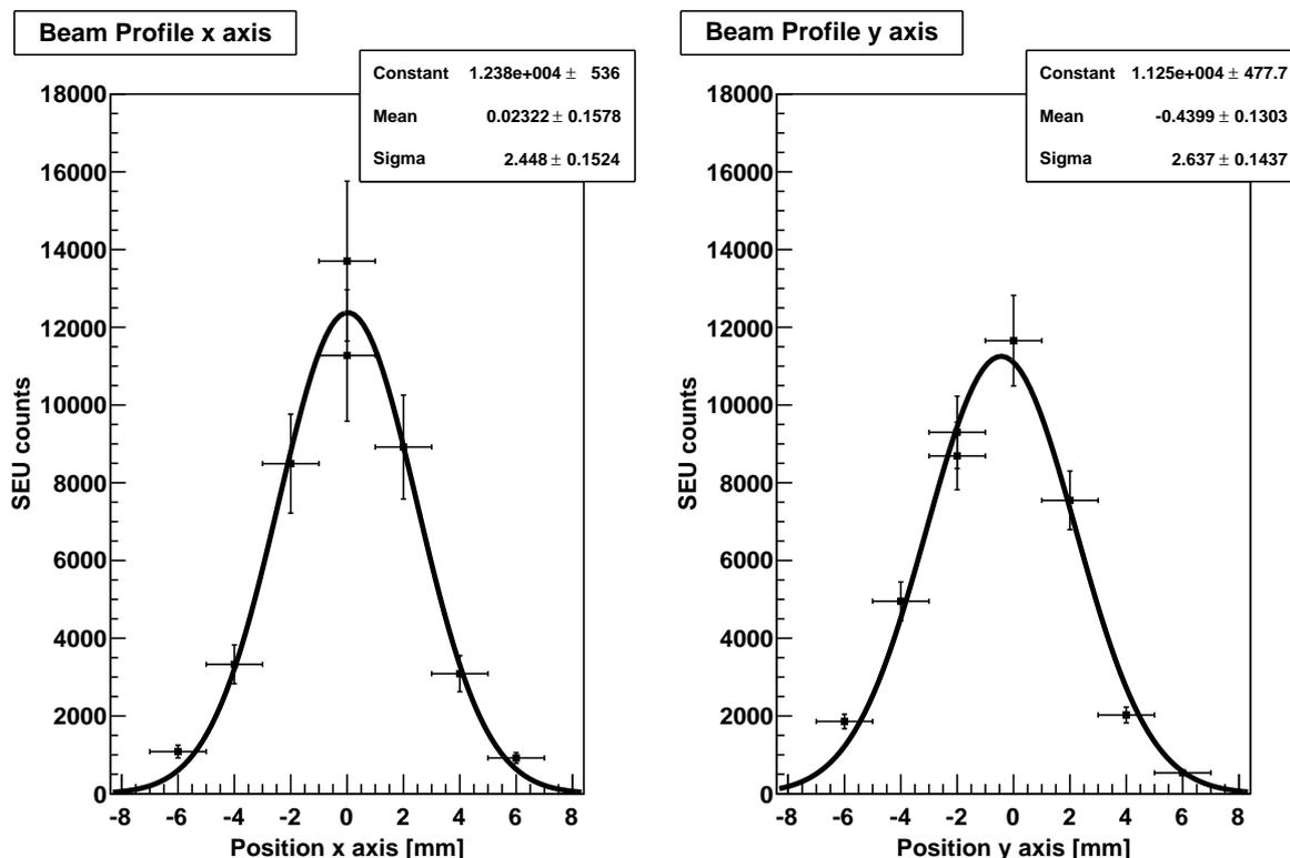
**Figure C.3:** The number of SEU counts at each position along the x- and y-axis fitted with a Gaussian fit. The uncertainty in the number of counts comes from fluctuations in the beam of 15%. The uncertainty in the position is due to the size of the laser point used for positioning. The Gaussian fit was created with ROOT [65].
