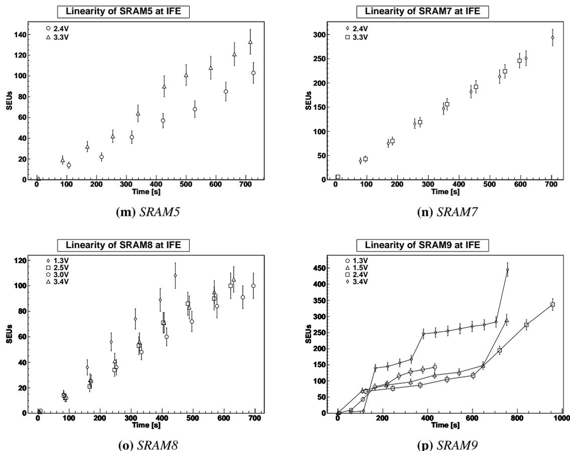
Figure 6.8: Linearity of devices tested at IFE. Lines added for clarity for SRAM3a and 9.
