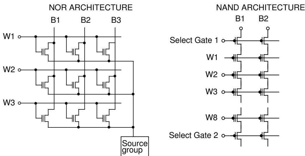
**Figure 3.9:** Schematic drawing of the flash NAND and NOR structures [16].
