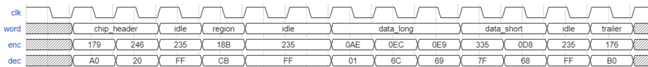
Figure 5.10: Wavediagram of an example ALPIDE data frame. In this particular frame only pixels within one region has been hit.
