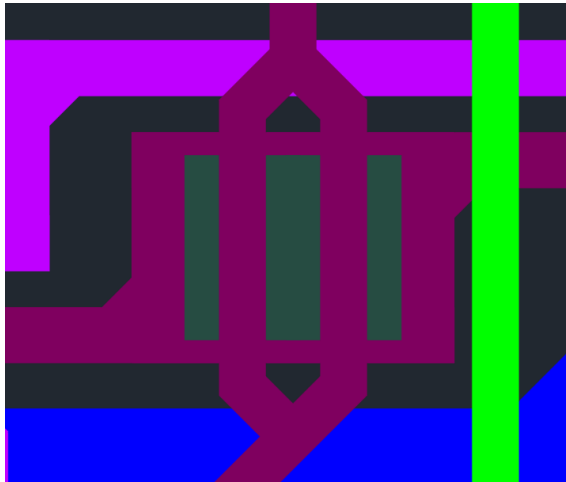
Figure 3.2: Illustration of a bond between the chip cable and the string flex. The vertical purple trace is on the chip cable flex, while the horizontal purple trace is on the string flex. The grey square marks the etching hole of the polyimide dielectric. This particular bond is for one of the differential traces of the slow control MLVDS-link. The size of the etching hole is roughly 500\ \mu\text{m}^2 . The double bond increases reliability.
