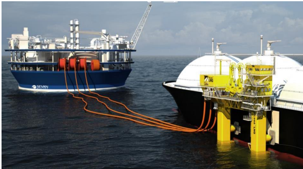
Figure 3-4: Offshore offloading concept for LNG from Cylindrical FPSO. The offloading vessel, "HiLoad" connects to the side of the receiving ship when loading LNG from the cylindrical FPSO [69].
