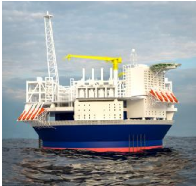
Figure 3-3: Cylindrical design of FPSO deployed in the sea by Sevan SSP. The model shows the topside and how the process equipment is distributed in several decks on the topside[45].
