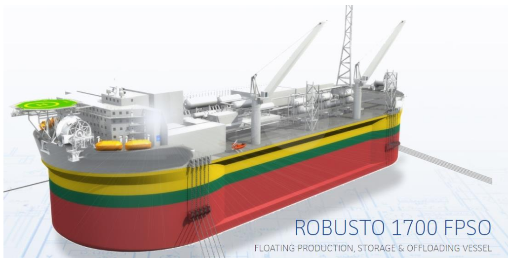
Figure 3-2: A ship-shaped FPSO by LMG Marin. The model shows the for act round fore-aft symmetric hull, mooring lines and topside, including accommodation, cranes, storage tanks etc. [44]
