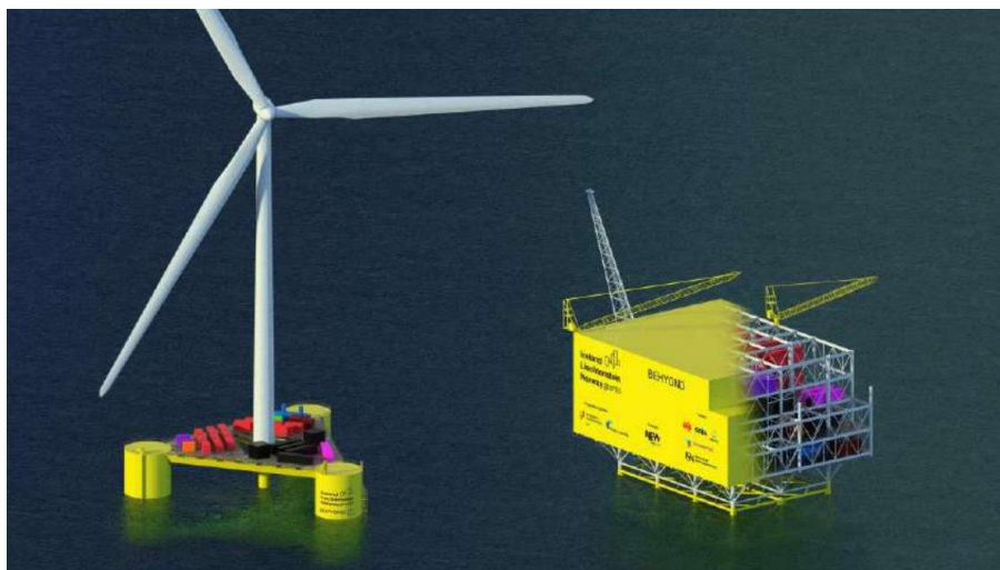
Figure 1-1: Difference between decentralised (left) and centralised (right) hydrogen production units [10].
