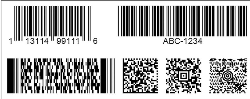
**Figure 3.** Examples of 1-D and 2-D code symbolisms: UPC-A and Code-39 (top), PDF417, Data Matrix, Aztec, and MaxiCode (bottom).
