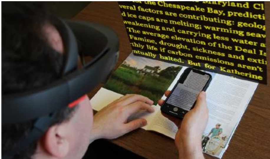
Figure 3: The AR HMD prototype used to magnify text in the study conducted by Stearns et al. (2018).
