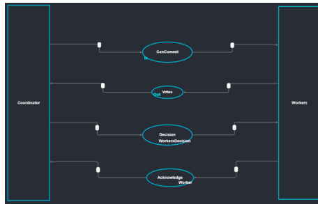
Figure 6.4: The two-phase commit protocol in our application with abstraction
