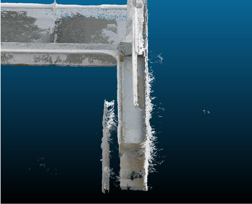
Figure 41: Flaring on railing from MLS
