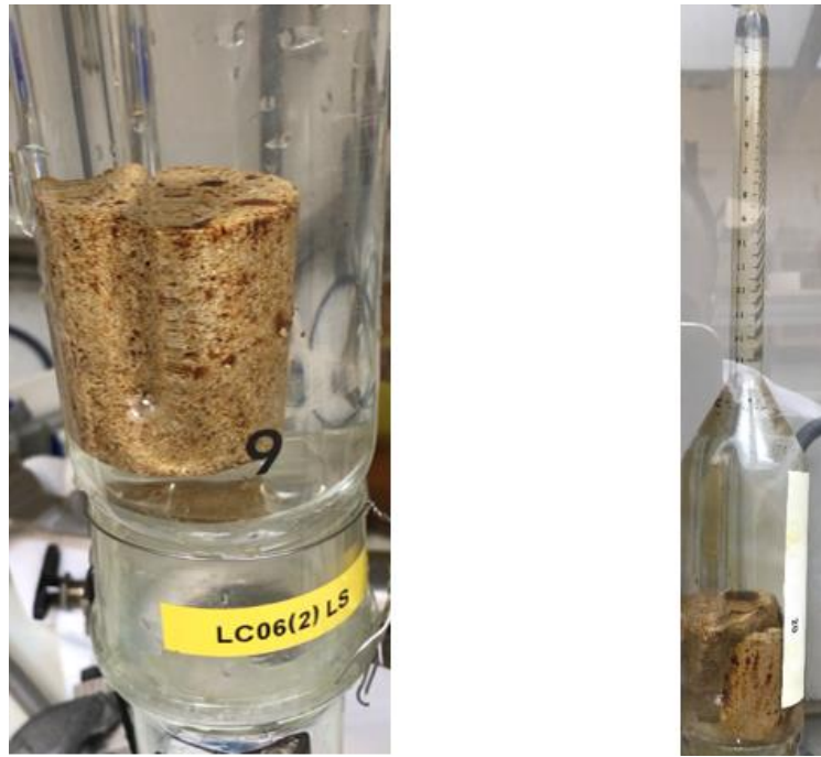
Figure 4.6: An example of spontaneous water imbibition of short cores. Notice that short core S2 was crushed (right)
