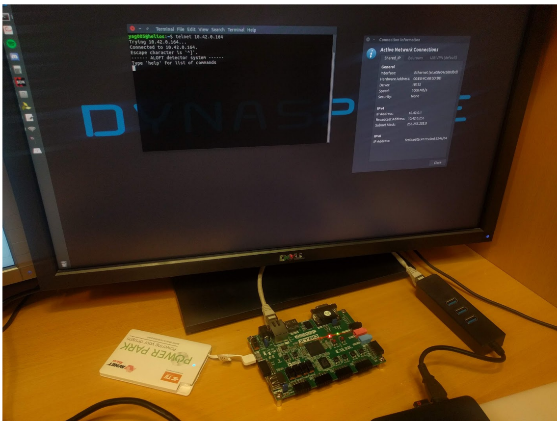
Figure 6.6: Test setup showing the Zybo board connected using a CAT6 ethernet, powered by a battery pack.
