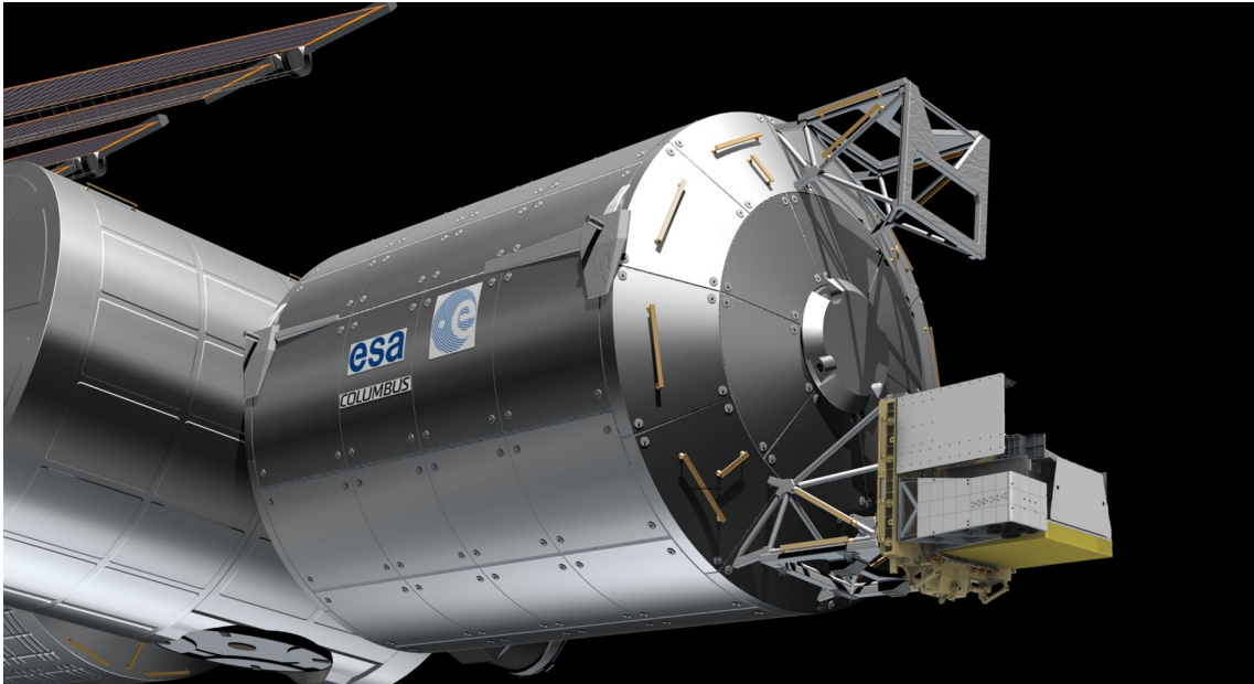
Figure 2.7: ASIM can be seen mounted on the far right of the Columbus module on the International Space Station in this illustration. Credits: ESA Concurrent Design Facility
