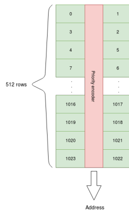
Figure 3.3: Pixel indexing by priority encoder inside a double column
