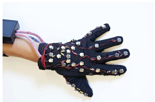
Figure 41 and 42. Press photos of the Mobile LORM glove . Left image shows how a user can input haptic data on the LORM glove. Right image shows how the user receives haptic output/feedback. Courtesy of developers.
