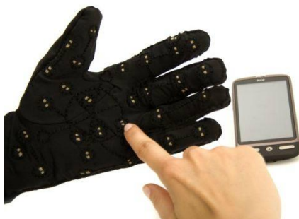
Figure 41 and 42. Press photos of the Mobile LORM glove . Left image shows how a user can input haptic data on the LORM glove. Right image shows how the user receives haptic output/feedback. Courtesy of developers.
