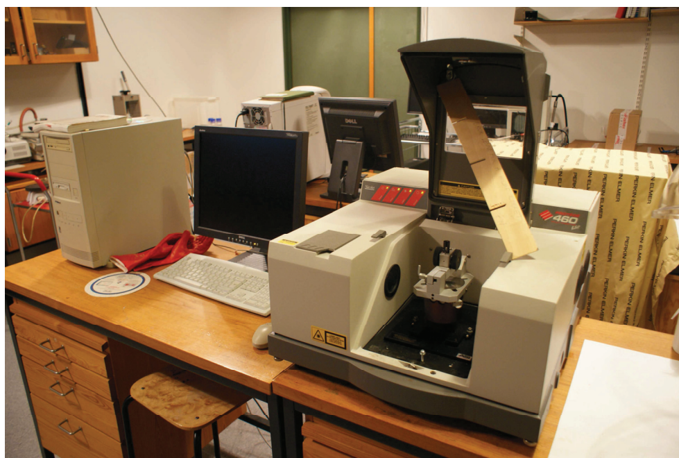
Figure 3.4: Nicolet Protegè 460 FT-IR spectrophotometer with an ATR measuring cell.
