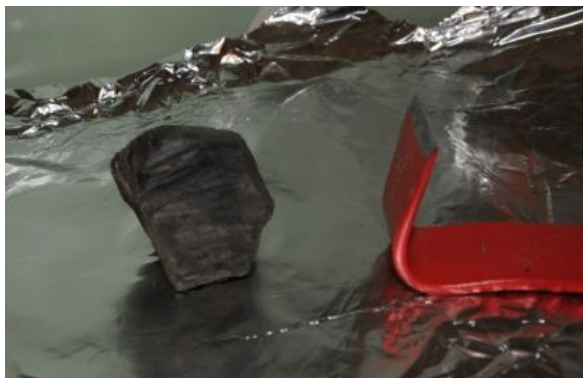
Figure 4: Sterile sub-sampling of the frozen permafrost core using a sterilised chisel on an aluminium foil covered bench in the freezing room (-20 °C).
